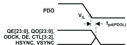
8-8. Delay From \overline{PDO} Low to Hi-Z Outputs
