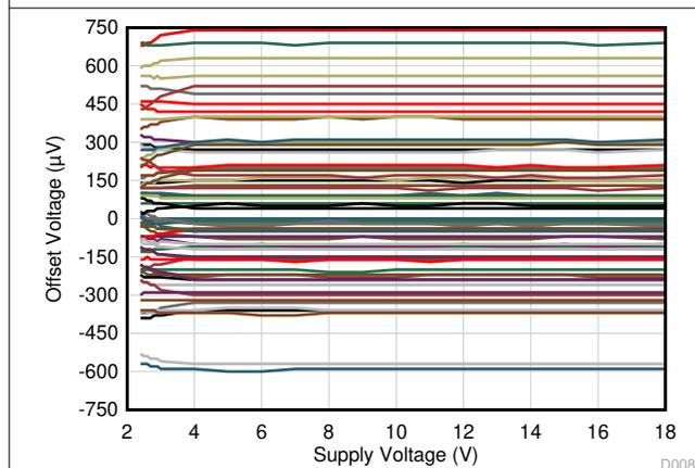
$V_{CM} = V_-$
