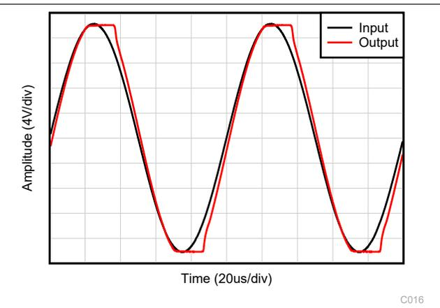
$V_{IN} = \pm 20\text{V}$ ,  $V_S = V_{OUT} = \pm 17\text{V}$
