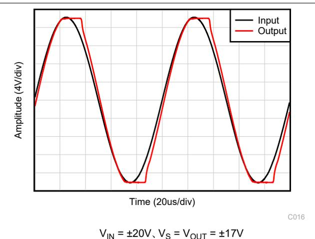
$V_{IN} = \pm 20\text{V}$ ,  $V_S = V_{OUT} = \pm 17\text{V}$
