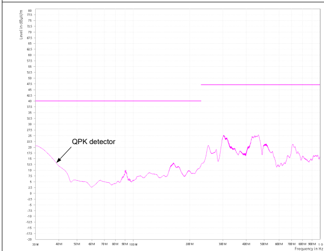
Figure 9-10. CISPR 32 Class B Radiated Emissions: Horizontal Polarization
