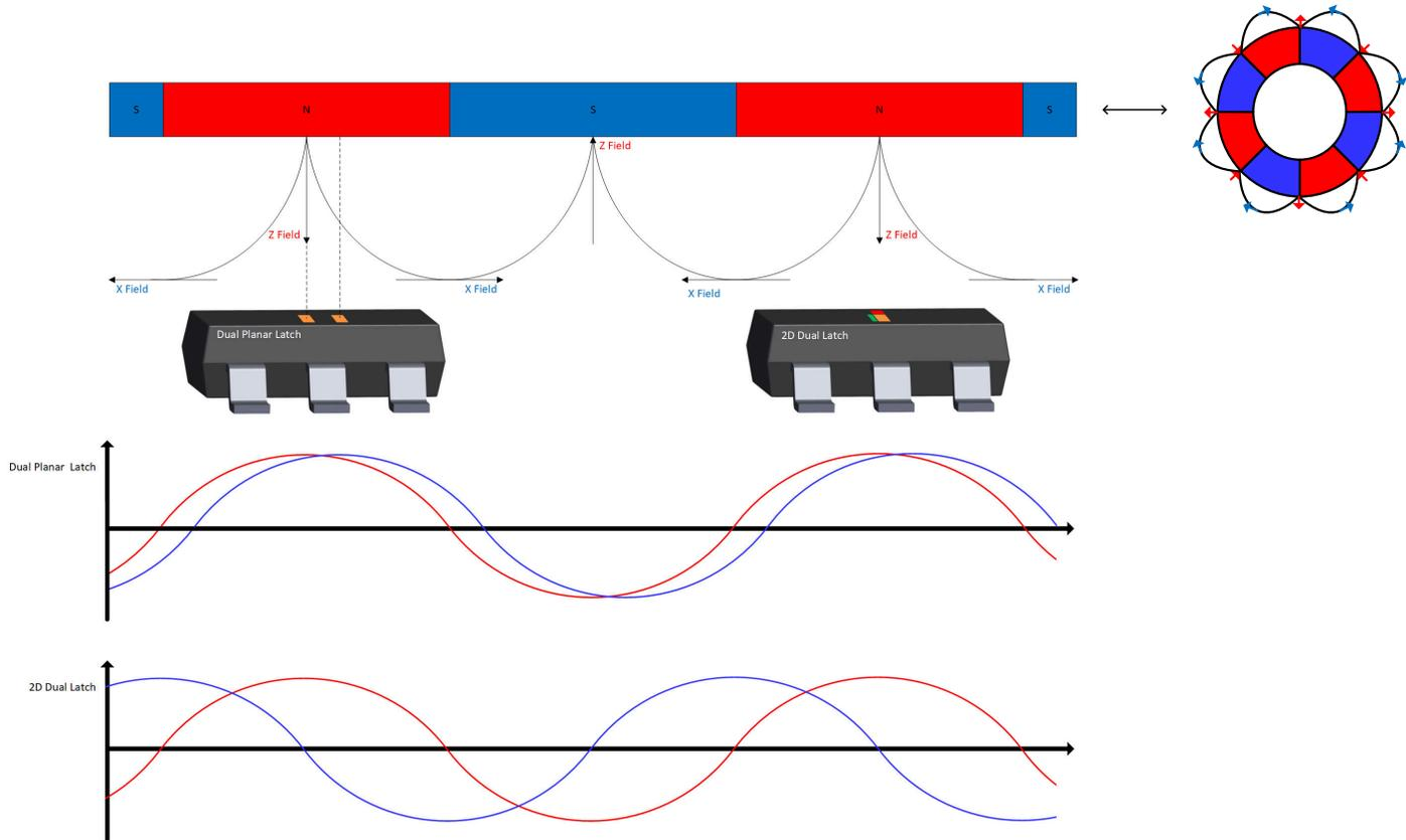
8-1. Dual Planar Latch vs. 2D Dual Latch
