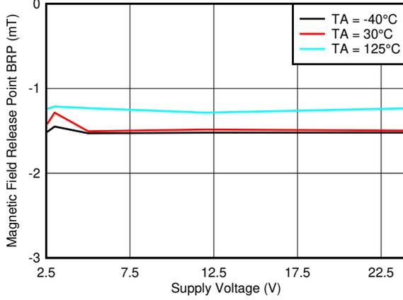
7-15. B<sub>RP\_Y</sub> Threshold vs. V<sub>CC</sub>
