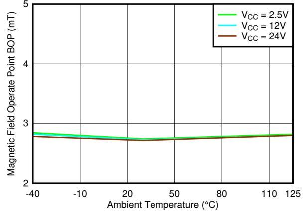
图 7-52. B<sub>OP\_Y</sub> Threshold vs. Temperature
