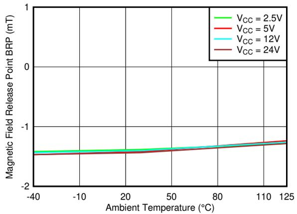
7-10. B<sub>RP\_X</sub> Threshold vs. Temperature
