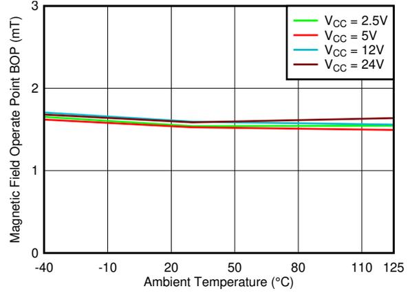
7-14. B<sub>OP\_Y</sub> Threshold vs. Temperature
