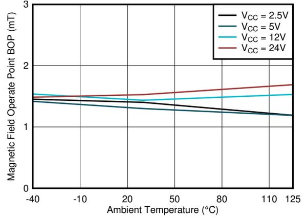
7-8. B<sub>OP\_X</sub> Threshold vs. Temperature
