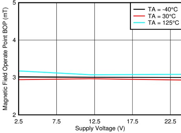
图 7-45. BOP\_X Threshold vs. VCC
