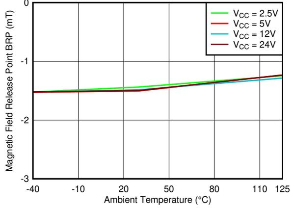
7-16. B<sub>RP\_Y</sub> Threshold vs. Temperature
