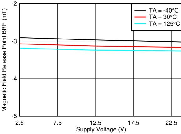
图 7-47. BRP\_X Threshold vs. VCC
