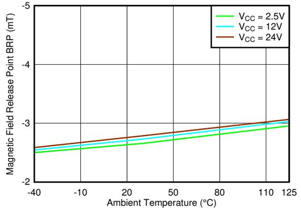
图 7-54. B<sub>RP\_Y</sub> Threshold vs. Temperature
