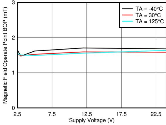
7-13. B<sub>OP\_Y</sub> Threshold vs. V<sub>CC</sub>
