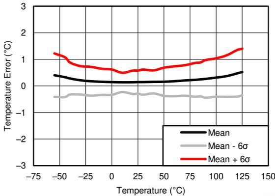
6-5. Temperature Error vs Temperature
