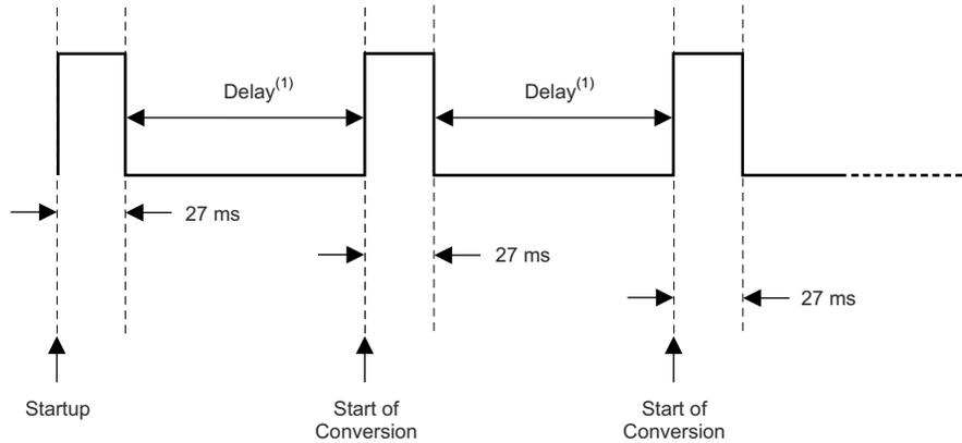
A. Delay is set by the CR bits in the configuration register.
