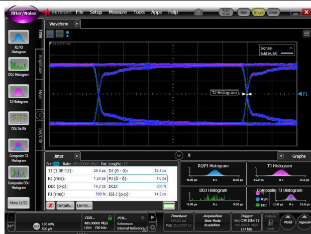
Figure 6-7. Through Calibration Traces at 480Mbps
