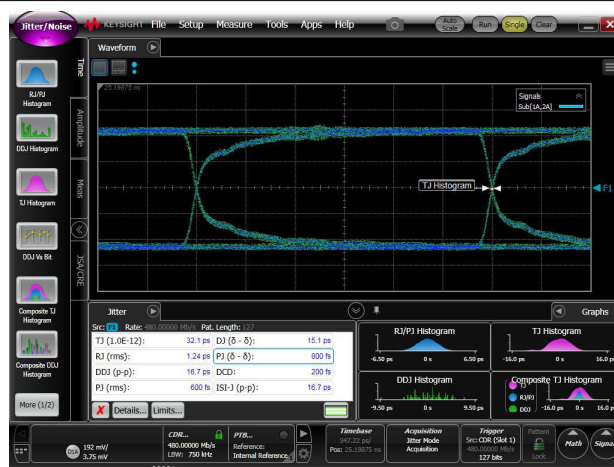
Figure 6-8. Through a Typical TMUXHS221LV Channel at 480Mbps
