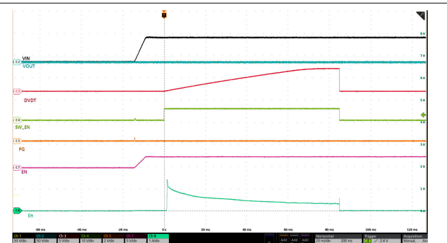
8-7. Power Up Into Short: V_{IN} = 54V , EN/UVLO Stepped Up From 0V to 3V
