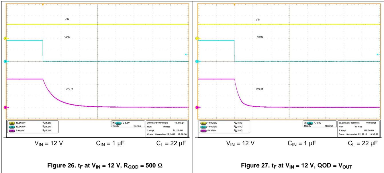
Figure 26.  $t_F$  at  $V_{IN} = 12\text{ V}$ ,  $R_{QOD} = 500\ \Omega$
