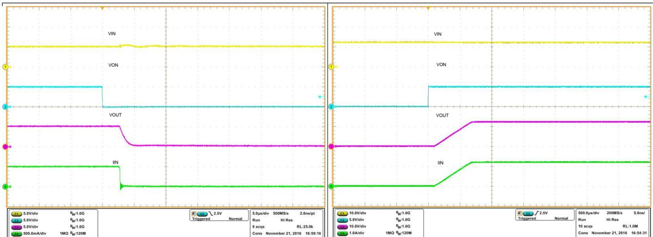
$V_{IN} = 5\text{ V}$        $C_{IN} = 1\text{ }\mu\text{F}$        $C_L = 0.1\text{ }\mu\text{F}$
