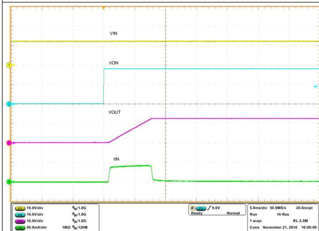
Figure 30. TPS22810 Inrush Current With  $C_L = 22\ \mu\text{F}$ ,  $CT = 27000\ \text{pF}$
