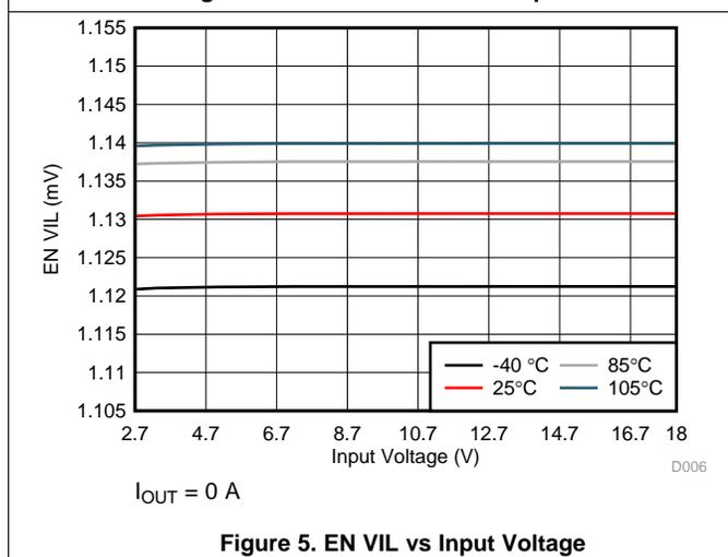
Figure 5. EN VIL vs Input Voltage
