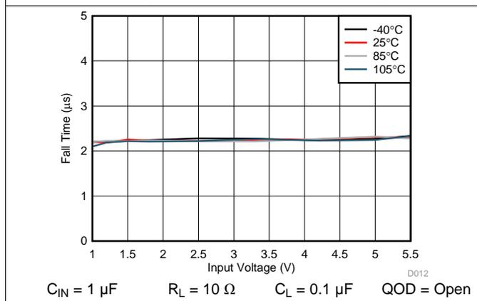
Figure 10. Fall Time vs Input Voltage
