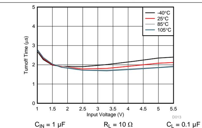
Figure 11. Turnoff Time vs Input Voltage
