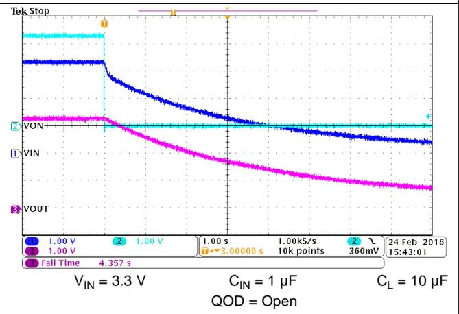
Figure 27. Fall Time ( $t_F$ ) at  $V_{IN} = 3.3 V$
