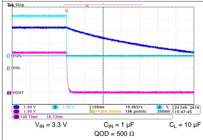
Figure 28. Fall Time ( $t_F$ ) at  $V_{IN} = 3.3 V$
