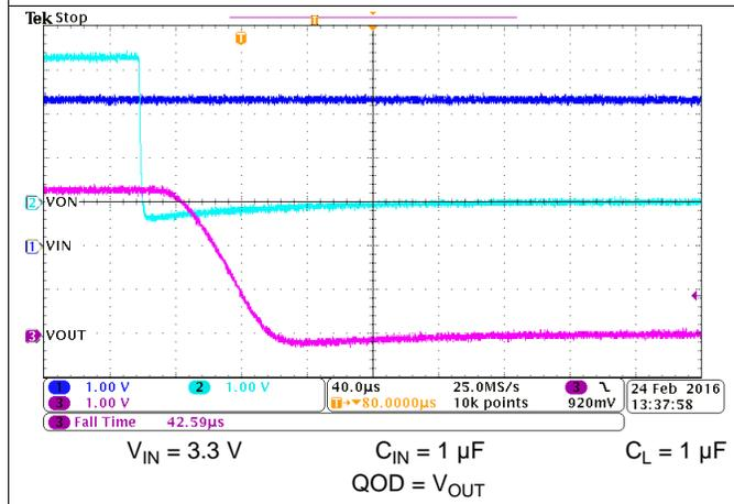
Figure 26. Fall Time ( $t_F$ ) at  $V_{IN} = 3.3 V$
