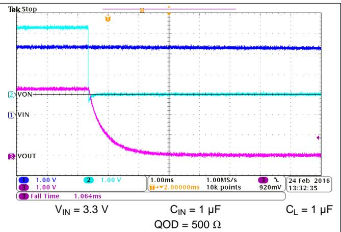
Figure 25. Fall Time ( $t_F$ ) at  $V_{IN} = 3.3 V$
