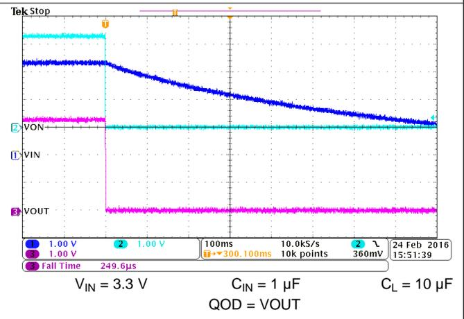
Figure 29. Fall Time ( $t_F$ ) at  $V_{IN} = 3.3 V$
