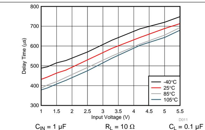
Figure 9. Delay Time vs Input Voltage
