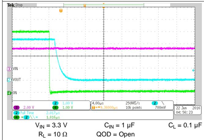
Figure 16. Fall Time ( $t_F$ ) at  $V_{IN} = 3.3\text{ V}$
