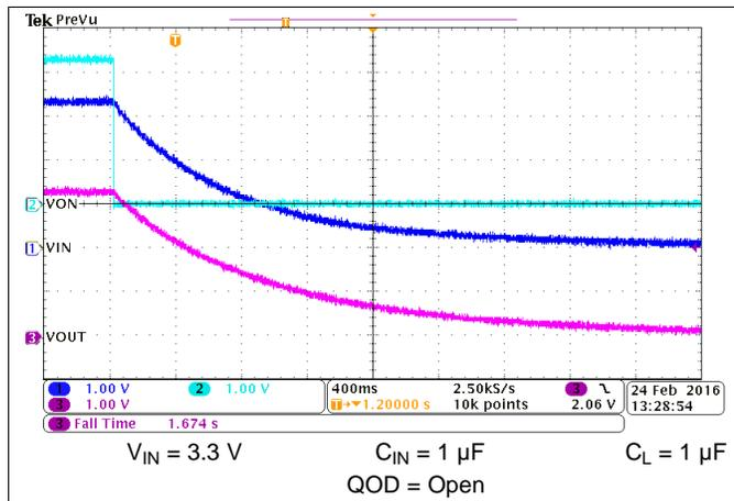
Figure 24. Fall Time ( $t_F$ ) at  $V_{IN} = 3.3 V$
