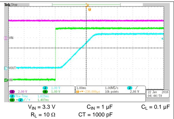
Figure 15. Rise Time ( $t_R$ ) at  $V_{IN} = 3.3\text{ V}$
