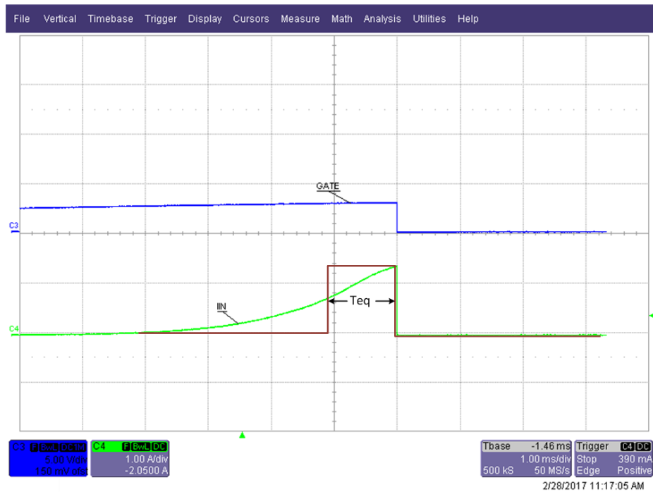
Figure 13. Teq During a Start Into a Short
