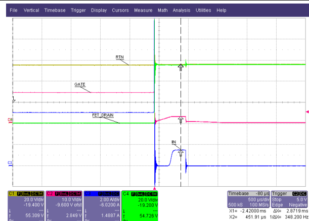
Scope GND = -48V_B, 5-A Load, After Inductor
