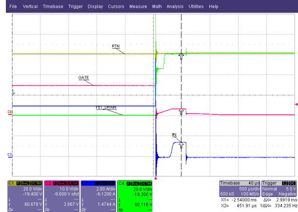
Scope GND = -48V_B, 5-A Load
