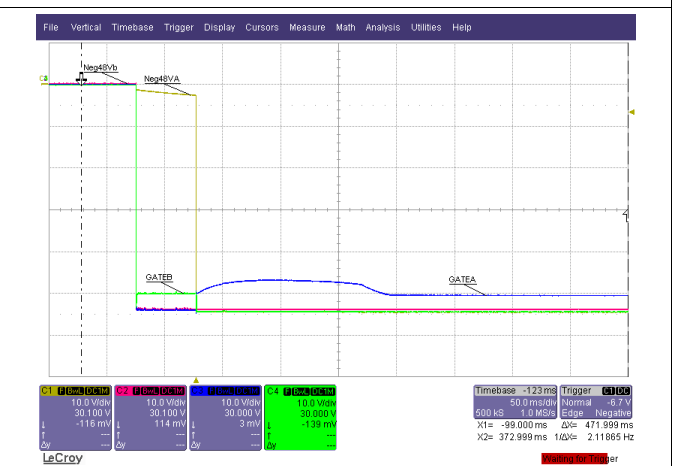
Figure 18. Start Up (Vin = 60 V)
