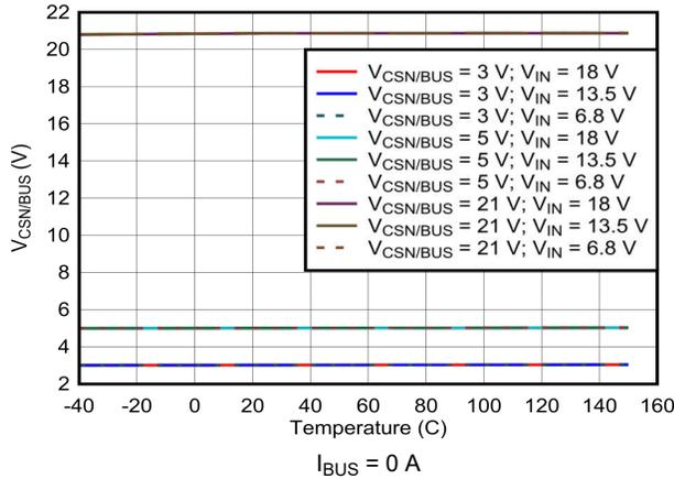
6-33. Buck-boost Output Voltage Regulation vs Temperature
