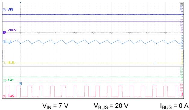
9-14. Boost Mode: Low  $V_{IN}$ , No Load
