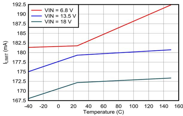
図 6-9. LDO\_5V Current Limit vs  $V_{IN}$  and Temperature
