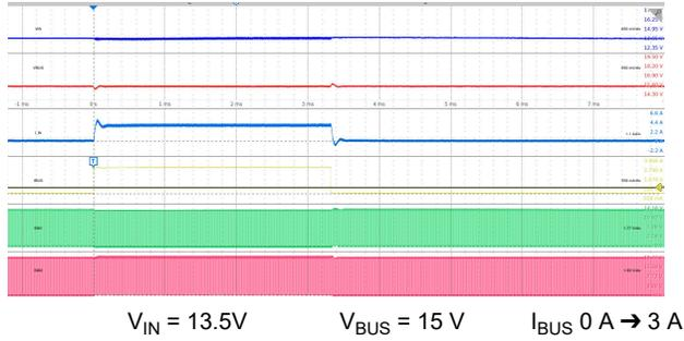
☒ 9-32. Load Transient (Buck-Boost):  $V_{BUS} = 15\text{ V}$
