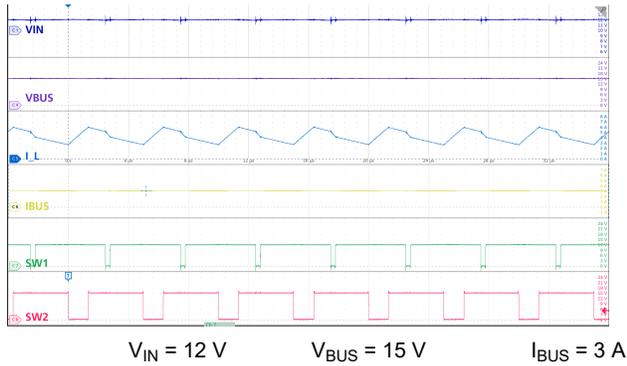
図 9-26. Buck-Boost Mode: Nominal  $V_{IN}$ , 3 A Load
