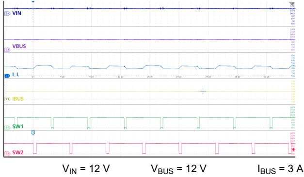
図 9-24. Buck-Boost Mode:  $V_{IN} = V_{BUS}$ , 3 A Load
