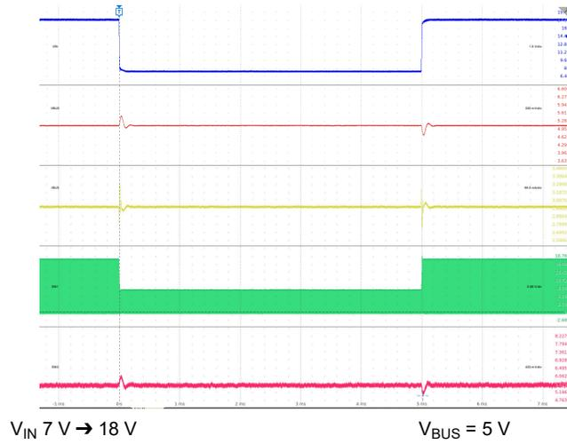
**図 9-38. Line Transient:  $V_{BUS} = 5\text{ V}$**
