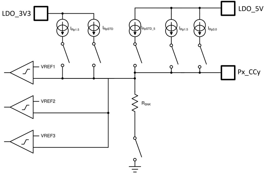
図 8-28. Plug and Orientation Detection Block
