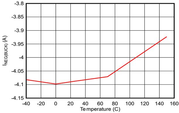
6-21. Buck Negative Current Limit vs Temperature
