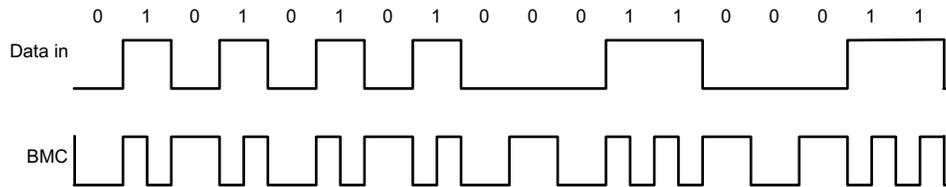
**Figure 8-22. Biphasic Mark Coding Example**
