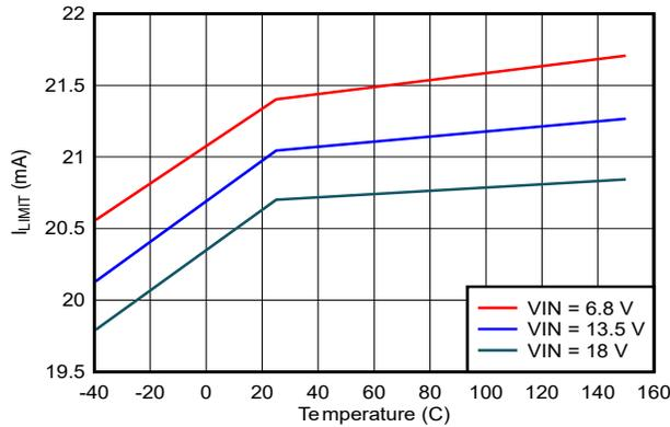
Figure 6-13. LDO\_1V5 Current Limit vs  $V_{IN}$  and Temperature
