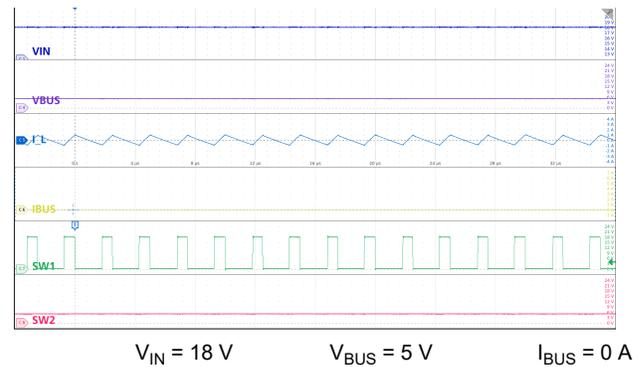
9-15. Buck Mode: High  $V_{IN}$ , No Load
