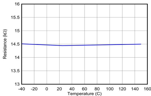
6-41. USB BC1.2: DM to AGND 15 k $\Omega$  Resistance,  $R_{DM\_DWN\_15k}$
