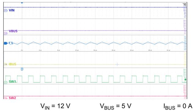
図 9-19. Buck Mode: Nominal  $V_{IN}$ , No Load
