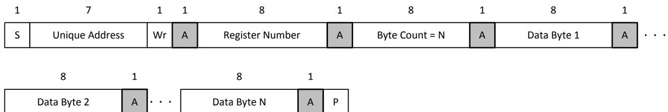
図 8-39. I<sup>2</sup>C Unique Address Write Register Protocol
