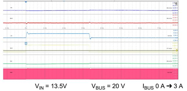
☒ 9-33. Load Transient (Boost):  $V_{BUS} = 20\text{ V}$
