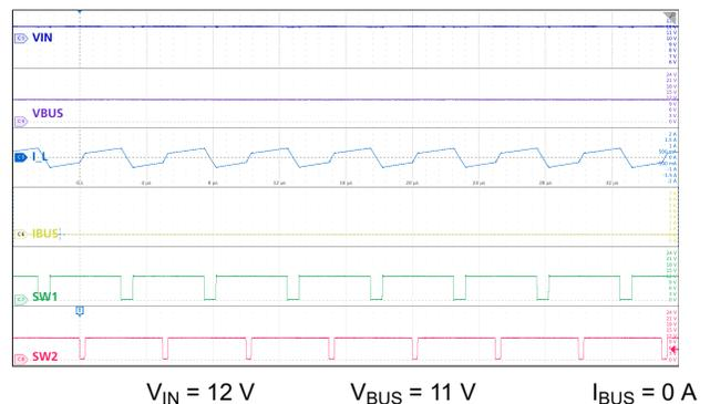
図 9-23. Buck-Boost Mode:  $V_{IN} > V_{BUS}$ , No Load
