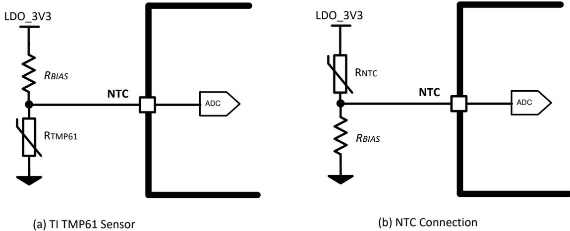
图 8-43. Thermistor Connections (a) PTC, (b) NTC
