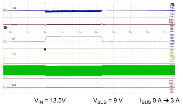
図 9-31. Load Transient (Buck):  $V_{BUS} = 9\text{ V}$
