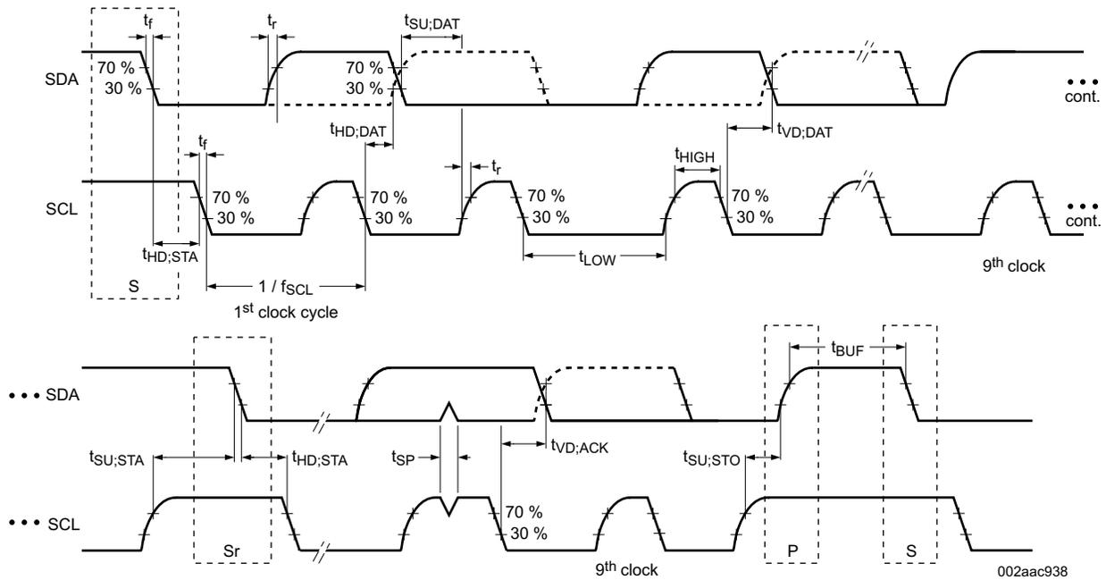
Figure 7-1. I<sup>2</sup>C Target Interface Timing
