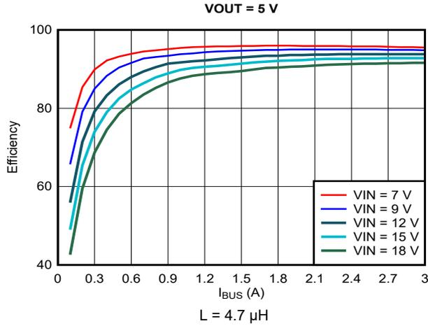
9-6. Efficiency vs Output Current ( $I_{OUT}$ ),  $V_{OUT} = 5$  V
