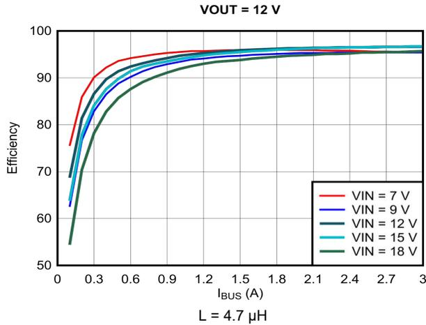
9-8. Efficiency vs Output Current ( $I_{OUT}$ ),  $V_{OUT} = 12$  V
