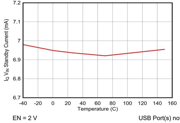
6-2.  $I_{Q\ V_{IN}}$  Standby Current vs Temperature
