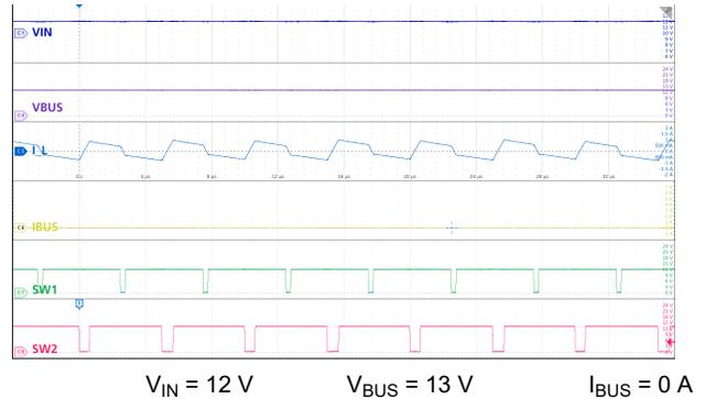
図 9-21. Buck-Boost Mode:  $V_{IN} < V_{BUS}$ , No Load
