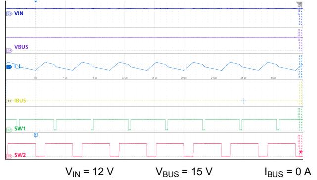
図 9-25. Buck-Boost Mode: Nominal  $V_{IN}$ , No Load
