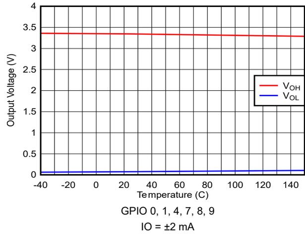
**6-44. GPIO: Output Voltage vs Output Current and Temperature**
