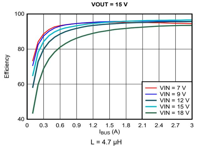
9-9. Efficiency vs Output Current ( $I_{OUT}$ ),  $V_{OUT} = 15$  V
