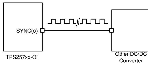
8-16. Using SYNC(o) to drive external DC/DC Converter
