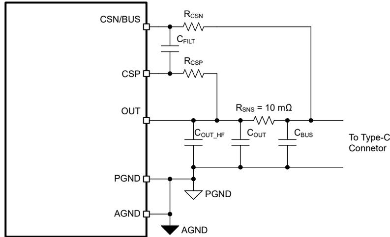
図 9-5. Current Sense Amplifier: RC Filter Components
