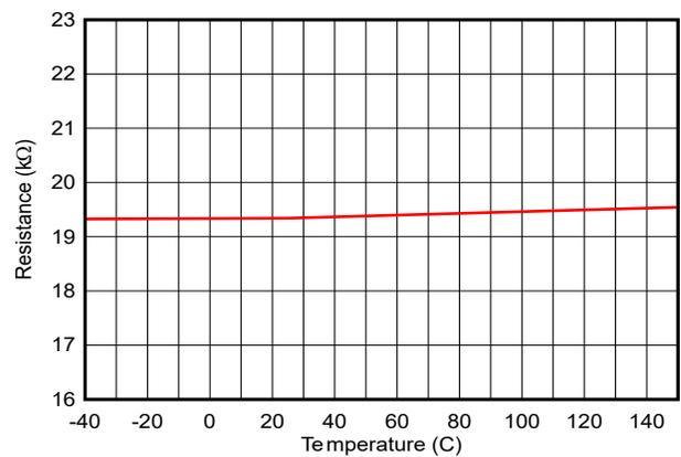
6-42. USB BC1.2: DM to AGND 20 k $\Omega$  Resistance,  $R_{DM\_DWN\_20k}$
