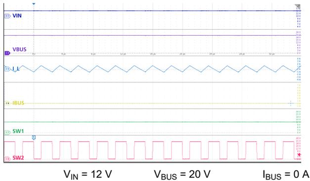
図 9-18. Boost Mode: Nominal  $V_{IN}$ , No Load
