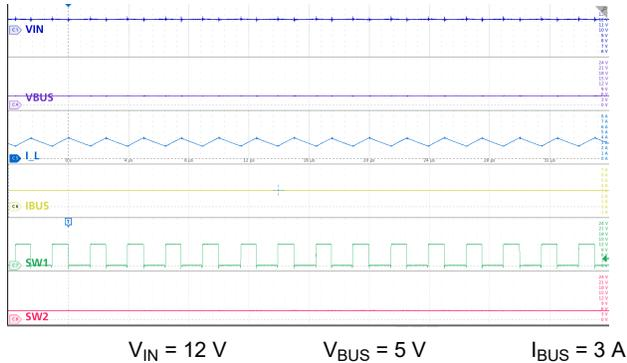
図 9-20. Buck Mode: nominal  $V_{IN}$ , 3 A Load
