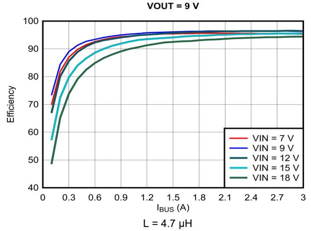
9-7. Efficiency vs Output Current ( $I_{OUT}$ ),  $V_{OUT} = 9$  V
