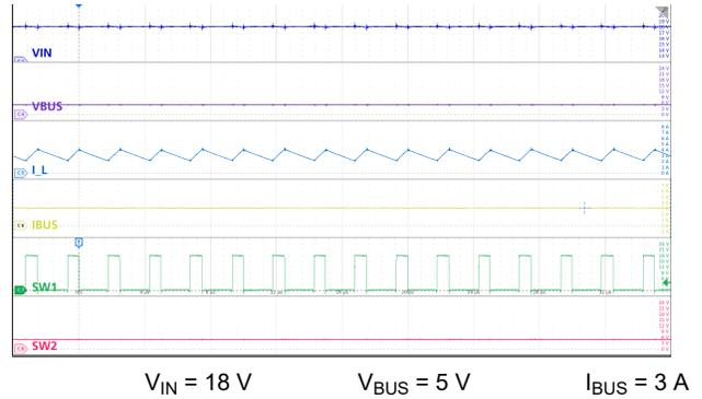
図 9-17. Buck Mode: High  $V_{IN}$ , 3 A load
