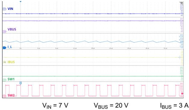
図 9-16. Boost Mode: Low  $V_{IN}$ , 3 A Load
