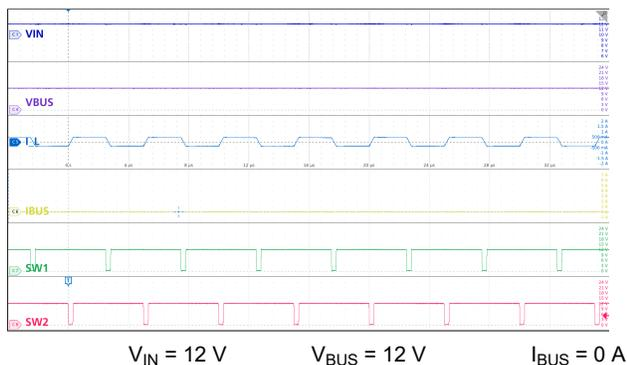
図 9-22. Buck-Boost Mode:  $V_{IN} = V_{BUS}$ , No Load
