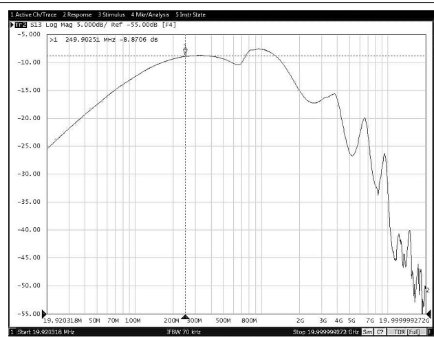
8-32. Off-State Data-Switch Isolation vs Frequency (TPS25830-Q1)
