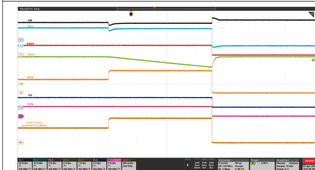
图 9-10. Circuit-Breaker Response: V_{IN} = 12 V, C_{TIMER} = 22 nF, C_{LOAD} = 50 mF, R_{IMON} = 200 \Omega , R_{IREF} = 40.2 k \Omega , and Load Current Stepped up From 250 A to 400 A for > 20 ms
