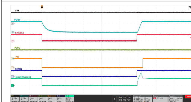
Input supply held steady, EN/UVLO pin toggled low and high
