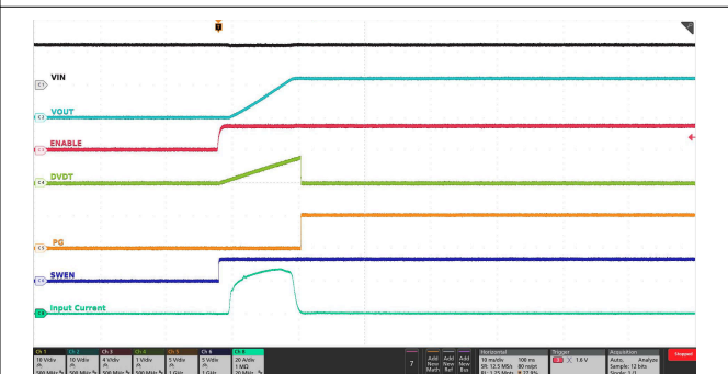
Input supply held steady, EN/UVLO pin toggled from low (below V_{SD(F)} ) to high (above V_{UVLO(R)} )
