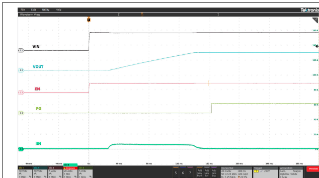
8-5. Input Hot Plug: V_{IN} Stepped Up from 0V to 12V, C_{LOAD} = 40\text{mF} , C_{DVDT} = 43\text{nF} , and R_{ILIM} on Each Device = 2k \Omega
