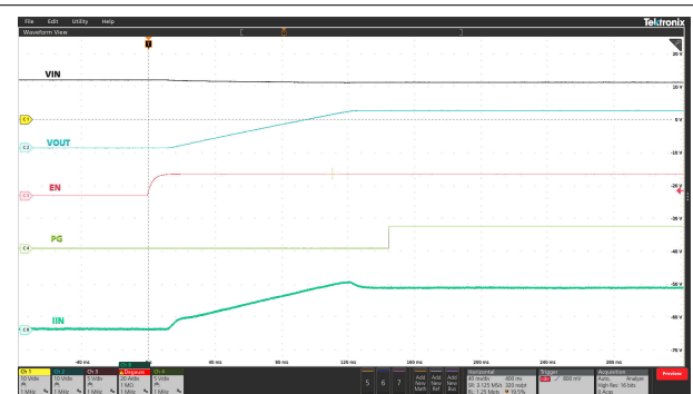
8-6. Start-up with EN/UVLO: V_{IN} = 12\text{V} , EN/UVLO Stepped Up From 0V to 3V, C_{LOAD} = 40\text{mF} , R_{LOAD(Start-up)} = 0.48\Omega , C_{DVDT} = 43\text{nF} , and R_{ILIM} on Each Device = 2k \Omega
