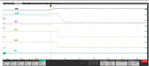
Input supply ramped up above V_{OVP(R)} .
