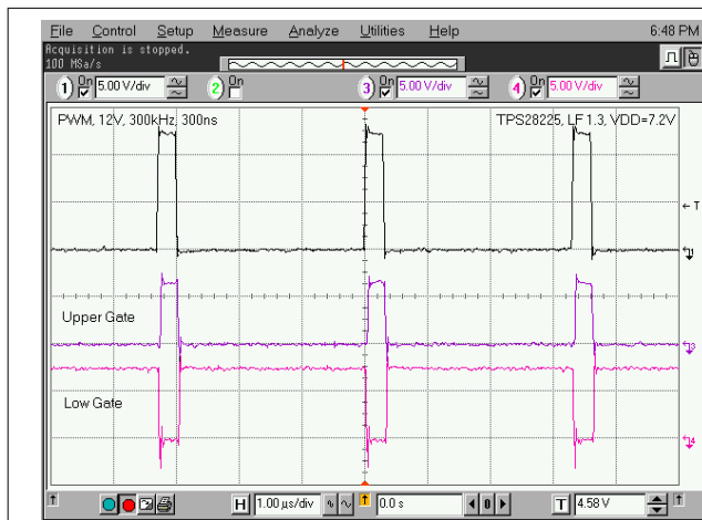
Figure 6-4. 12-V PWM Pulse at V_{DD} = 7.2\text{ V}
