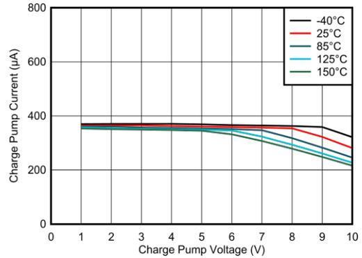
5-4. Charge Pump Current vs Charge Pump Voltage
