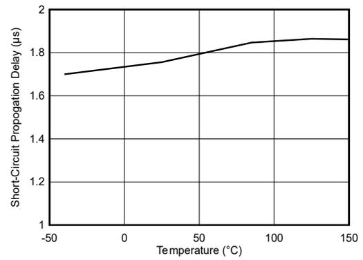
Figure 5-8. Short-Circuit Protection Response Time ( $t_{(SC)}$ ) vs Temperature
