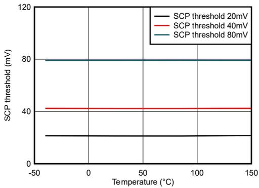
Figure 5-7. Short-Circuit Threshold ( $V_{(SCP/LWU)}$ ) vs Temperature
