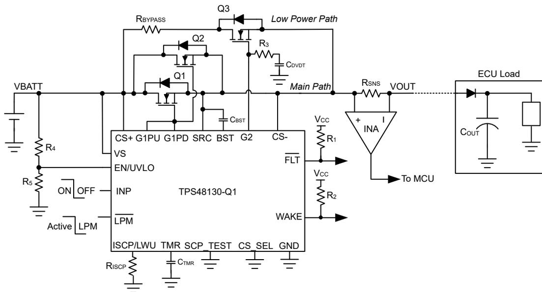
**図 8-13. Always ON Automotive E-fuse With Bi-directional Current Sensing and Software I<sup>2</sup>t**
