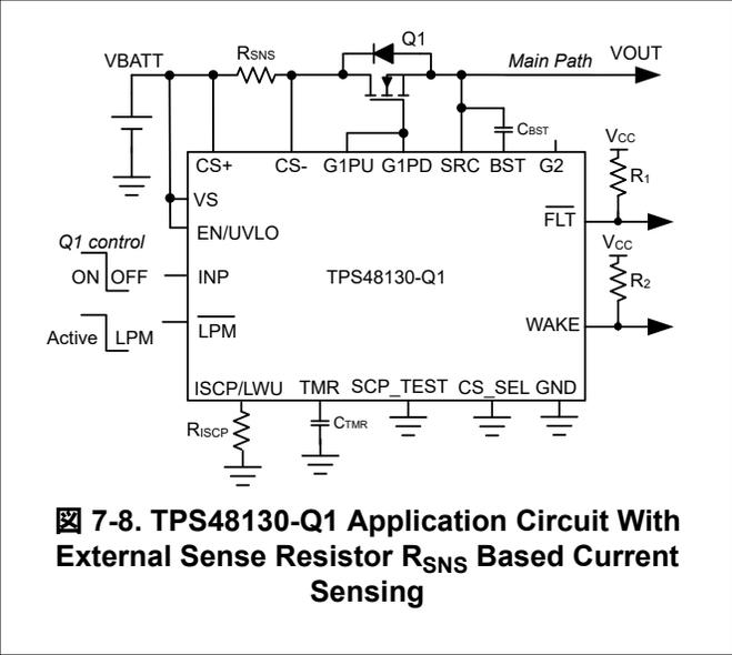
Set the hard short-circuit detection threshold using an external  $R_{ISCP}$  resistor across ISCP/LWU and GND pins. Use 式 8 to calculate the required  $R_{ISCP}$  value:
