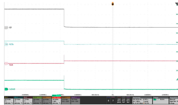
図 8-8. Latch-Off Response of TPS4813-Q1 for an Overcurrent Fault
