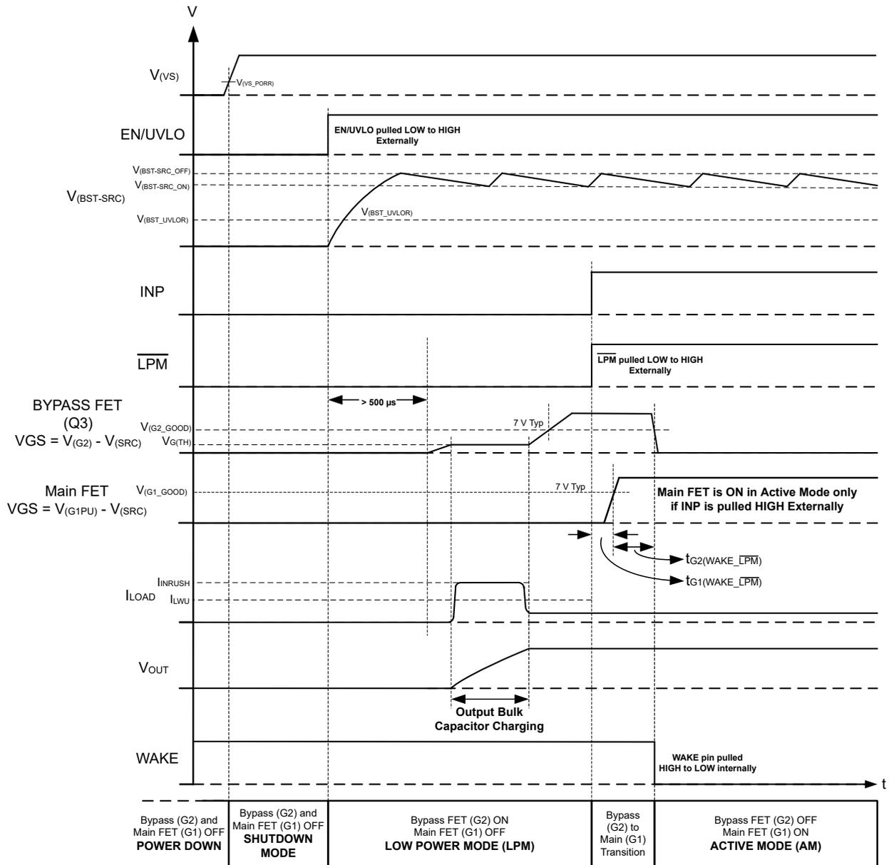
7-14. State Transition Timing Diagram With LPM Trigger
