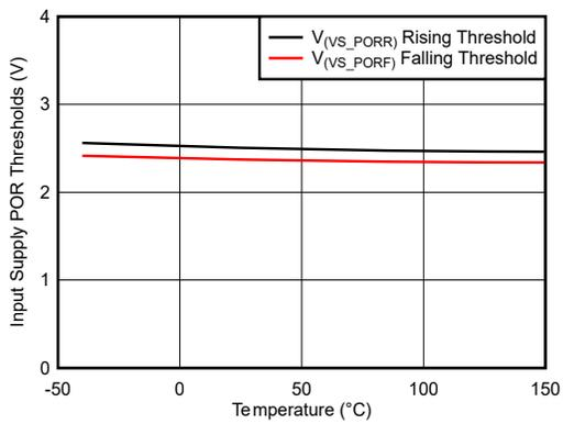
Figure 5-9. Input Supply POR Thresholds vs Temperature
