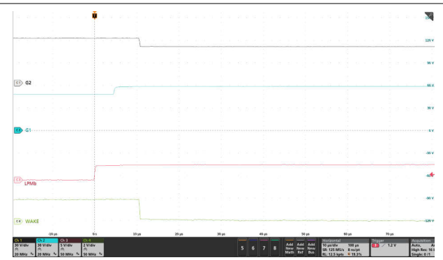
図 8-5. State Transition From LPM to Active Mode (LPM = Low to High, VIN = 48V, No Load)
