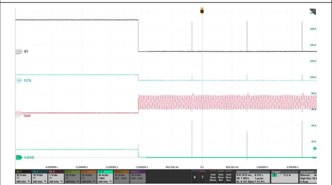
**図 8-7. Auto-Retry Response of TPS4813-Q1 for an Overcurrent Fault**
