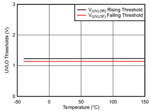
Figure 5-10. Input Supply UVLO Thresholds vs Temperature
