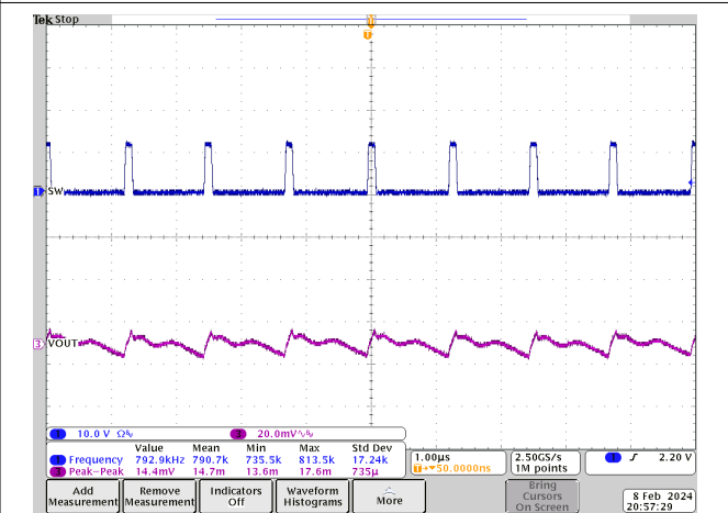
図 7-15. Output Voltage Ripple, 800kHz FFCM, No load, PVIN = 12V, VOUT = 1.1V
