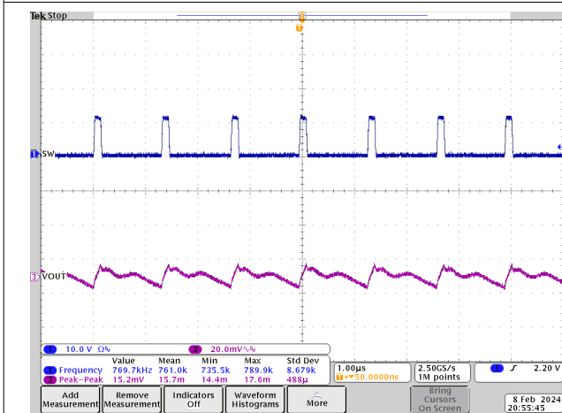
図 7-14. Output Voltage Ripple, 800kHz FFCM, 40A Load, PVIN = 12V, VOUT = 1.1V
