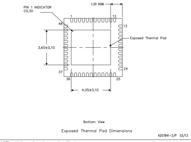
NOTE: All linear dimensions are in millimeters
