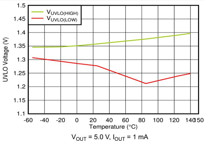
6-41. UVLO Rising and Falling Threshold vs Temperature
