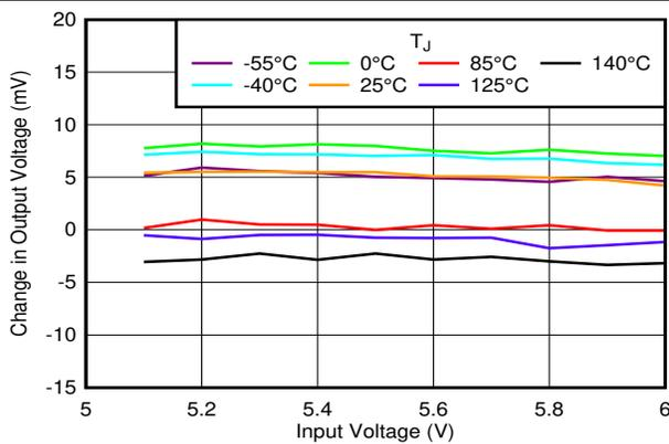
$V_{OUT} = 5.0\text{ V}$ ,  $I_{OUT} = 1\text{ mA}$
