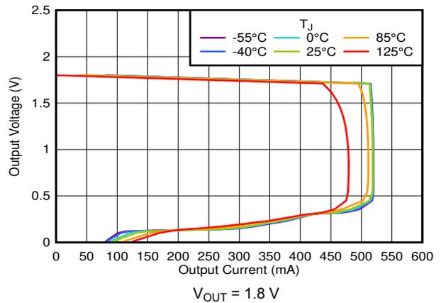
6-38. Foldback Current Limit vs  $I_{OUT}$  and Temperature
