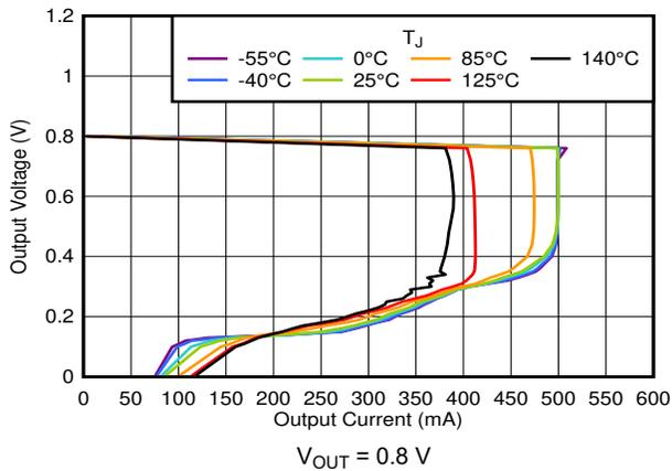
6-37. Foldback Current Limit vs  $I_{OUT}$  and Temperature
