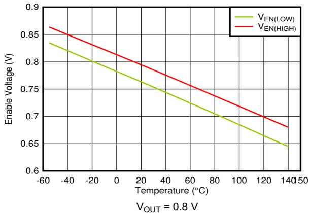
6-39. EN High and Low Threshold vs Temperature
