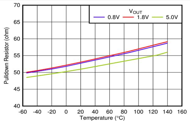
6-42. Pulldown Resistor vs Temperature and  $V_{OUT}$
