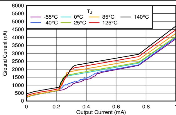
$V_{OUT} = 1.8\text{ V}$ ,  $V_{IN} = V_{EN} = 2.3\text{ V}$
