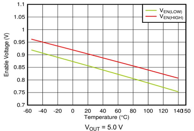
6-40. EN High and Low Threshold vs Temperature
