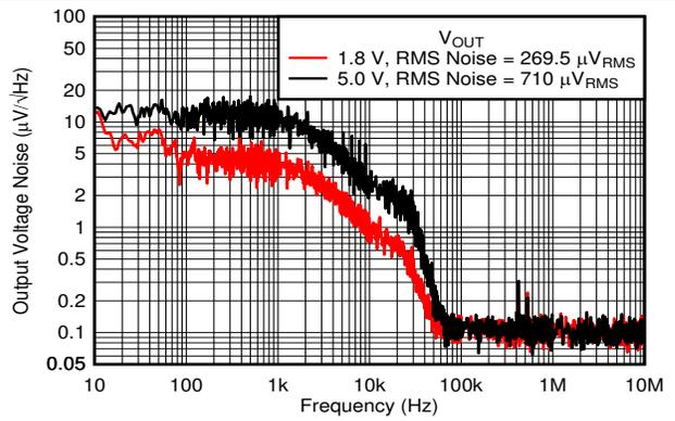
6-48. Output Noise vs Frequency and  $V_{OUT}$
