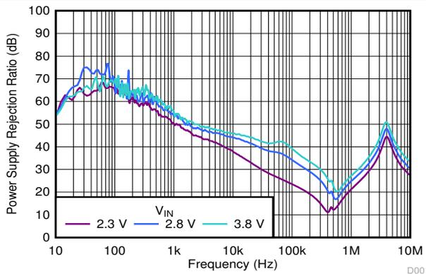
6-47. PSRR vs Frequency and  $V_{IN}$
