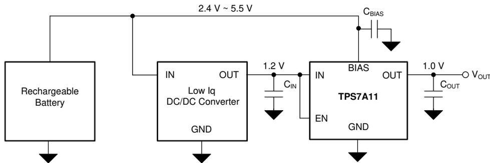
图 8-4. High Efficiency Supply From a Rechargeable Battery
