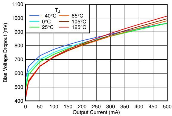
Figure 6-7.  $V_{BIAS}$  Dropout vs  $I_{OUT}$  and Temperature
