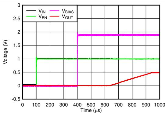
**6-17. Startup With  $V_{BIAS}$  Powering Up After  $V_{IN}$  and  $V_{EN}$**
