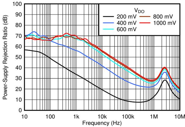
$C_{IN} = 0\text{ }\mu\text{F}$ ,  $V_{OUT} = 1.0\text{ V}$ ,  $I_{OUT} = 500\text{ mA}$ ,  $V_{DO} = V_{IN} - V_{OUT}$
