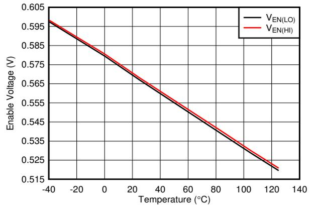
6-32. Enable High and Low Threshold vs Temperature
