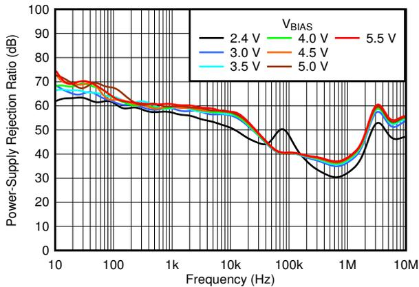
$C_{IN} = 2.2\text{ }\mu\text{F}$ ,  $V_{OUT} = 1.0\text{ V}$ ,  $I_{OUT} = 500\text{ mA}$ ,  $C_{BIAS} = 0\text{ }\mu\text{F}$
