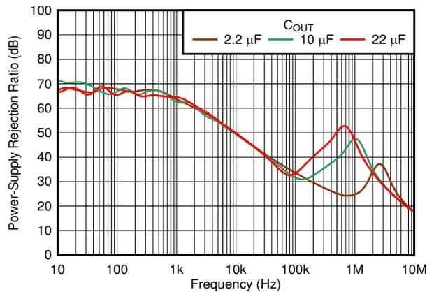
$C_{IN} = 0\text{ }\mu\text{F}$ ,  $V_{OUT} = 1.0\text{ V}$ ,  $I_{OUT} = 500\text{ mA}$
