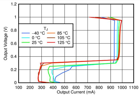
6-12. Foldback Output Current Limit vs  $I_{OUT}$  and Temperature
