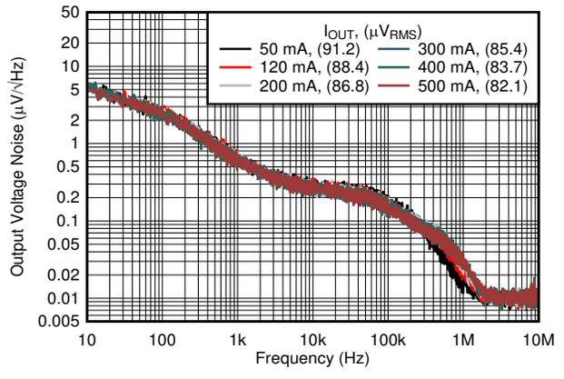
$V_{OUT} = 1.0\text{ V}$
