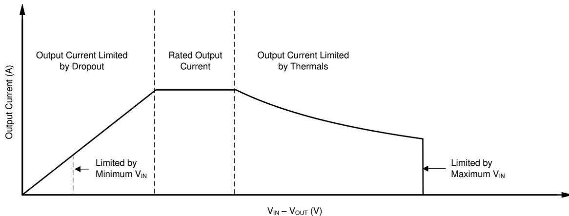
图 8-3. Continuous Operation Diagram With Description of Regions
