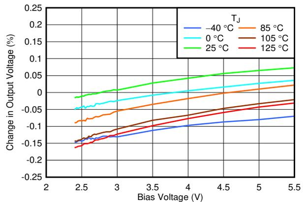
6-6. Output Accuracy vs  $V_{BIAS}$  and Temperature
