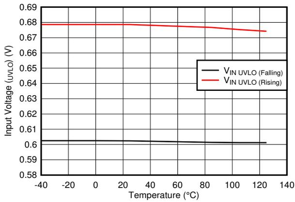
6-31.  $V_{UVLO(IN)}$  Rising and Falling Threshold vs Temperature
