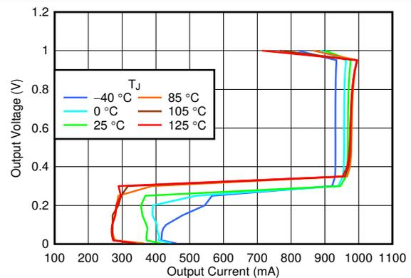
Figure 6-12. Foldback Output Current Limit vs  $I_{OUT}$  and Temperature
