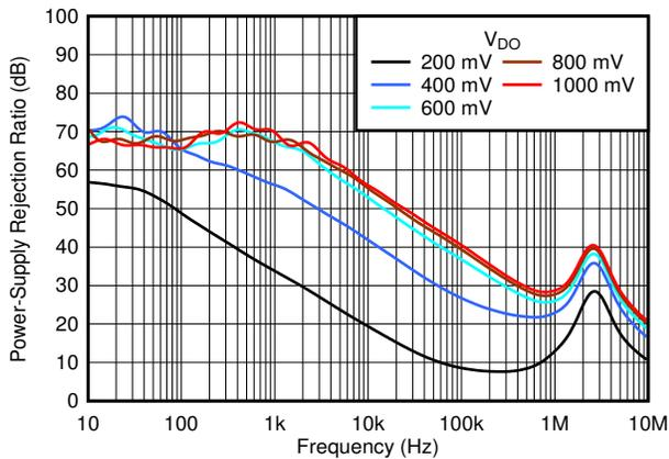
$C_{IN} = 0\text{ }\mu\text{F}$ ,  $V_{OUT} = 1.0\text{ V}$ ,  $I_{OUT} = 500\text{ mA}$ ,  $V_{DO} = V_{IN} - V_{OUT}$
