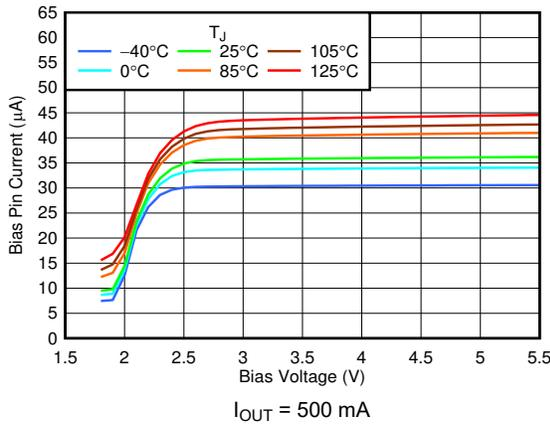
6-9.  $I_{Q(BIAS)}$  vs  $V_{BIAS}$  and Temperature
