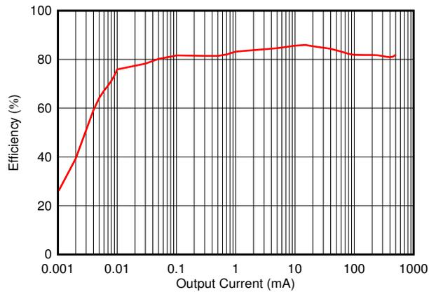
$$V_{IN} = V_{EN} = 1.2 \text{ V}, C_{IN} = 2.2 \text{ } \mu\text{F}, V_{OUT} = 1.0 \text{ V}, C_{OUT} = 2.2 \text{ } \mu\text{F}, V_{BIAS} = 2.4 \text{ V}, C_{BIAS} = 0.1 \text{ } \mu\text{F}$$
