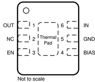
TI recommends connecting the SON (DRV) package thermal pad to ground.
