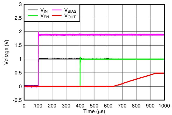
**6-16. Startup With Separated  $V_{EN}$**
