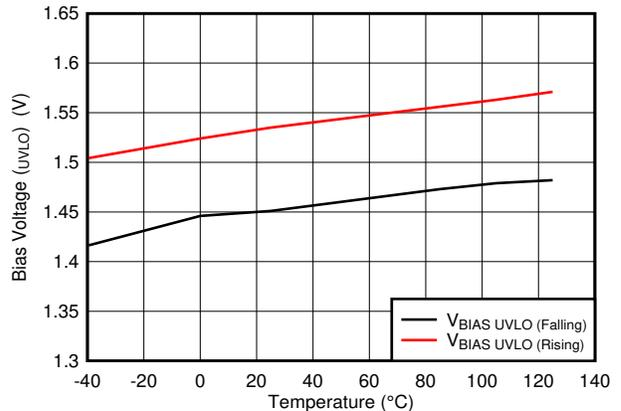
6-30.  $V_{UVLO(BIAS)}$  Rising and Falling Threshold vs Temperature
