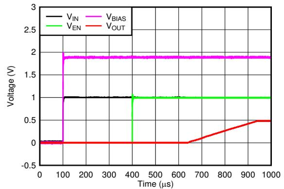
**6-16. Startup With Separated  $V_{EN}$**
