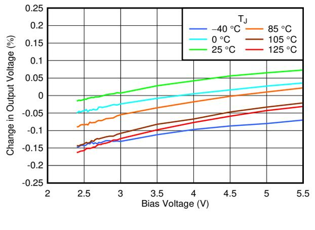
6-6. Output Accuracy vs  $V_{BIAS}$  and Temperature
