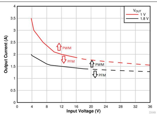
**Figure 7-15. PFM/PWM Thresholds (1 V and 1.8 V)**
