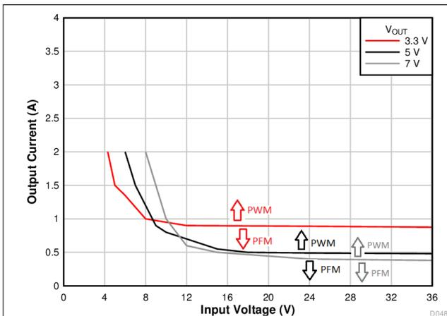
**Figure 7-14. PFM/PWM Thresholds (3.3 V, 5 V, and 7 V)**
