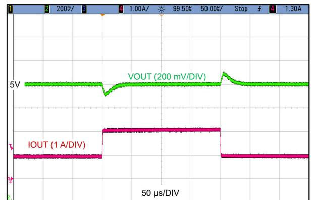
$V_{IN} = 24\text{ V}$        $V_{OUT} = 5\text{ V}$        $f_{SW} = 1\text{ MHz}$
