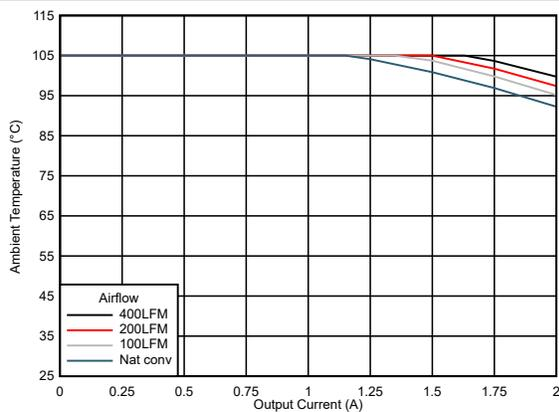
The device is soldered to a 64-mm × 83-mm, 4-layer PCB.
