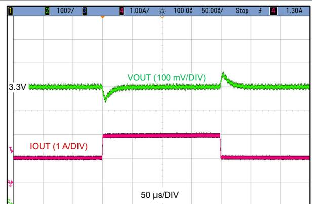
$V_{IN} = 24\text{ V}$        $V_{OUT} = 3.3\text{ V}$        $f_{SW} = 1\text{ MHz}$
