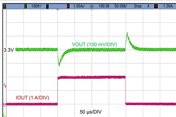
$V_{IN} = 24\text{ V}$        $V_{OUT} = 3.3\text{ V}$        $f_{SW} = 1\text{ MHz}$
