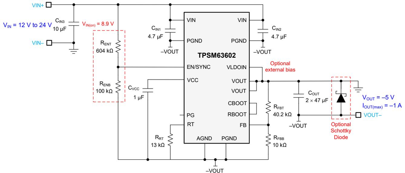
Figure 9-12. Circuit Schematic
