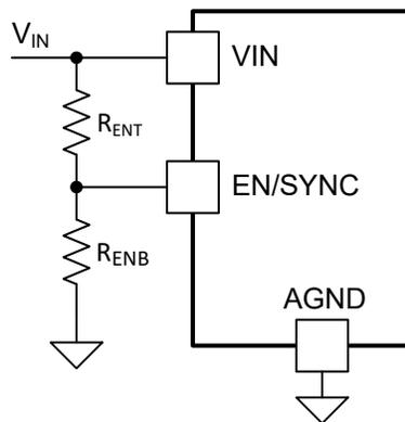
**Figure 8-3.  $V_{IN}$  UVLO Using the EN/SYNC Pin**
