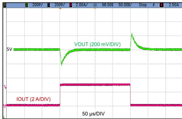
$V_{IN} = 24\text{ V}$        $V_{OUT} = 5\text{ V}$        $f_{SW} = 1\text{ MHz}$
