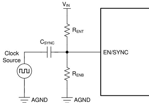
**Figure 8-4. Typical Synchronization Using the EN/SYNC Pin**
