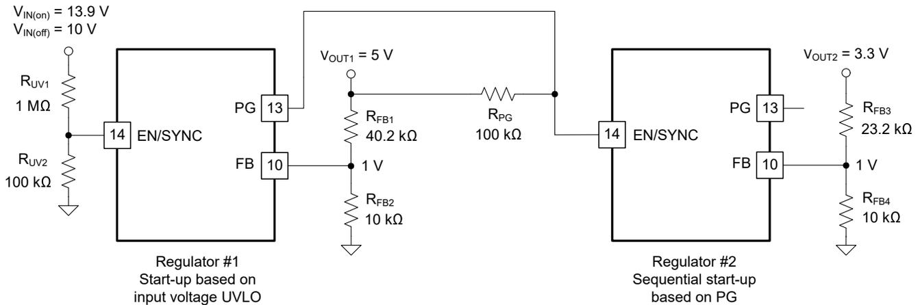
**Figure 8-6. TPSM63602 Sequencing Implementation Using PG and EN/SYNC**
