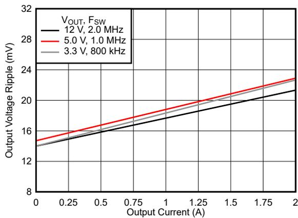
$C_{OUT} = 2 \times 47\text{-}\mu\text{F}$  ceramic, 25-V, 1206 case size
