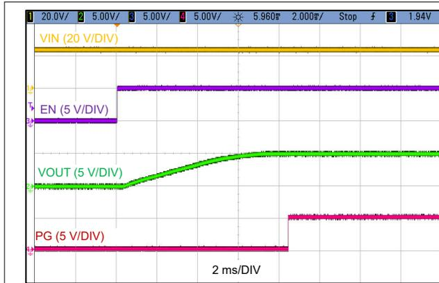
$V_{IN} = 24\text{ V}$        $V_{OUT} = 5\text{ V}$
