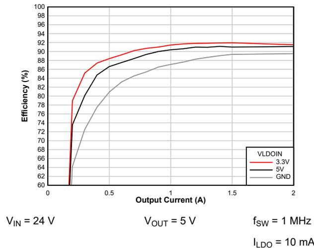
Figure 8-8. Efficiency Improvements with VLDOIN (V<sub>OUT</sub> = 5 V)
