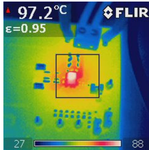
図 7-9. Case Temperature, V_{IN} = 24V , I_{OUT} = 3A , f_{sw} = 1000kHz
