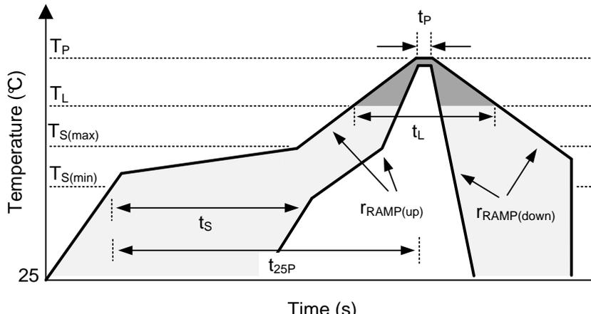
shows the recommended reflow-oven thermal profile. Proper post-assembly cleaning is also critical to device performance. Refer to [Power Module MSL Ratings and Reflow Ratings](#) for more information.
