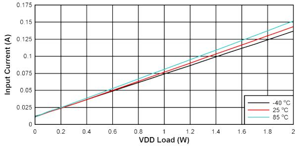
⊠ 10-20. Input Current vs Load on  $V_{DD-VEE}$ :  $V_{IN} = 24\text{ V}$ ,
