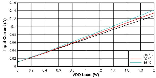
⊠ 10-21. Input Current vs Load on  $V_{DD-VEE}$ :  $V_{IN} = 27\text{ V}$ ,
