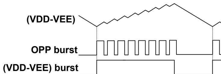
图 11-4. Diagram of Over-Power-Protection with baby burst
