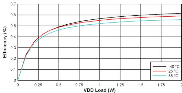
10-16. Efficiency vs Load on  $V_{VDD-VEE}$ :  $V_{IN} = 21\text{ V}$ ,  $V_{VDD-VEE} = 22\text{ V}$ ,  $V_{COM-VEE} = 4\text{ V}$ , No Load on  $V_{COM-VEE}$
