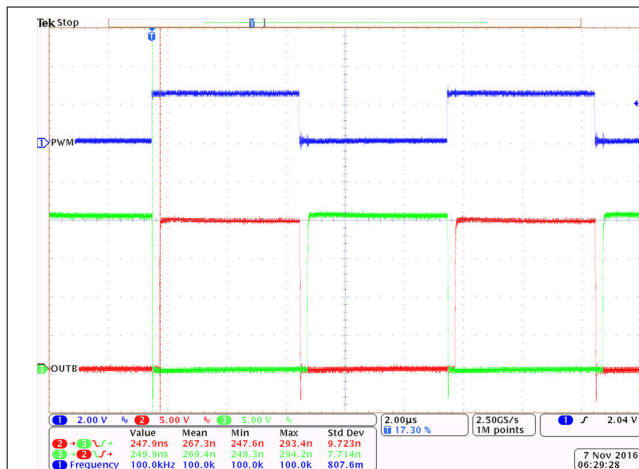
Figure 9-5. Bench Test Waveform for PWM and OUTA/B
