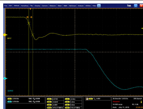
図 9-13. PWM Input (yellow) and Driver Output (blue) Falling Edge
