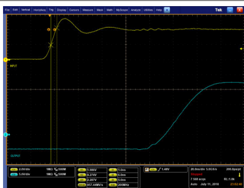
図 9-12. PWM Input (yellow) and Driver Output (blue) Rising Edge
