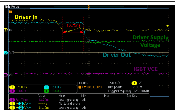
7-3. UCC27524A Used to Drive IGBT in the Boost Converter
