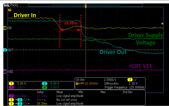
図 7-3. UCC27624 Used to Drive IGBT in the Boost Converter
