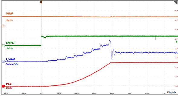
図 6-25. Start-Up with En/FLT From Low to High: VINP = 5.0V , VCC = 5.0V , 18Ω Load
