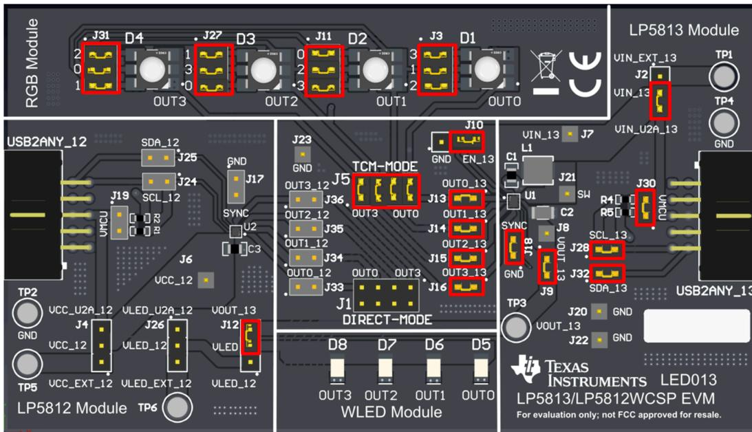
Figure 3-3. 4-Scan Mode and Enable Boost without External Power supply
