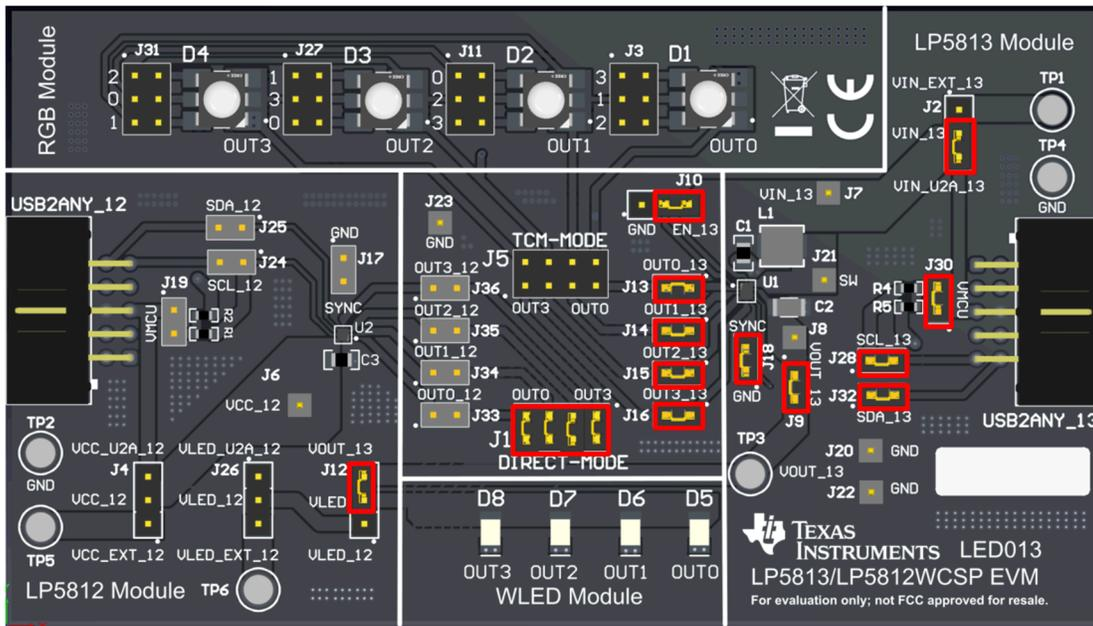
**Figure 3-5. Direct mode and Enable Boost without External Power supply**
