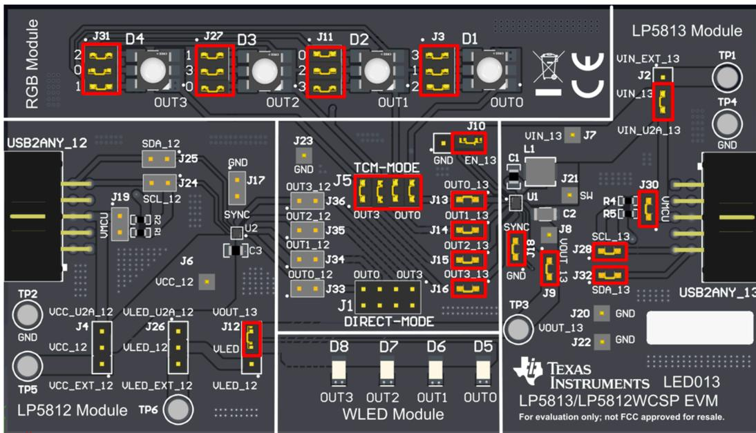
Figure 3-2. 4-Scan Mode and Enable Boost without External Power supply
