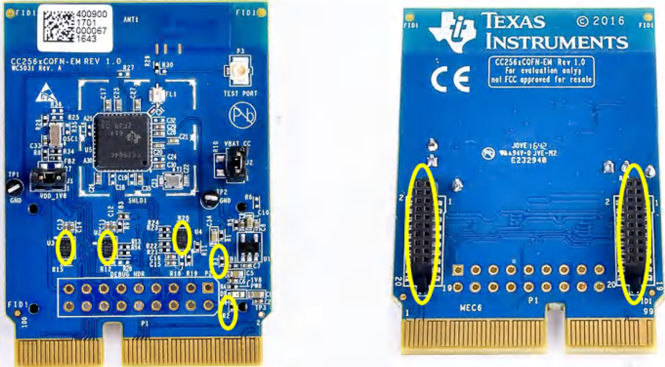
Figure 3-4. CC256XCQFN-EM Hardware Modifications for COM Connector
