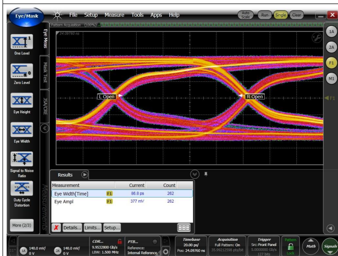
Figure 9. 5 Gbps Source Eye Diagram
