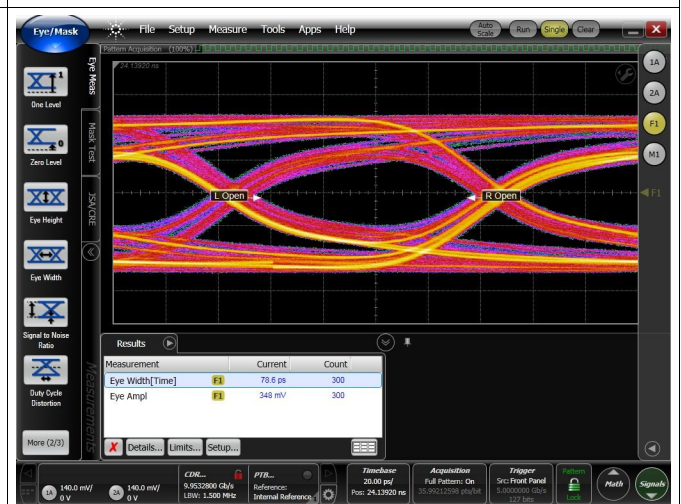
Figure 10. 5 Gbps Output Eye Diagram
