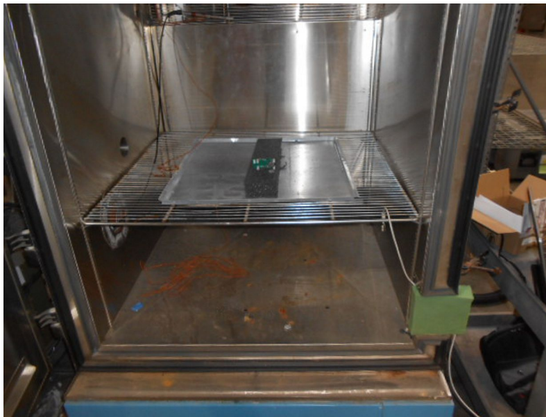
図 19. Wireless PIR Motion Detector Temperature and Humidity Test Setup
