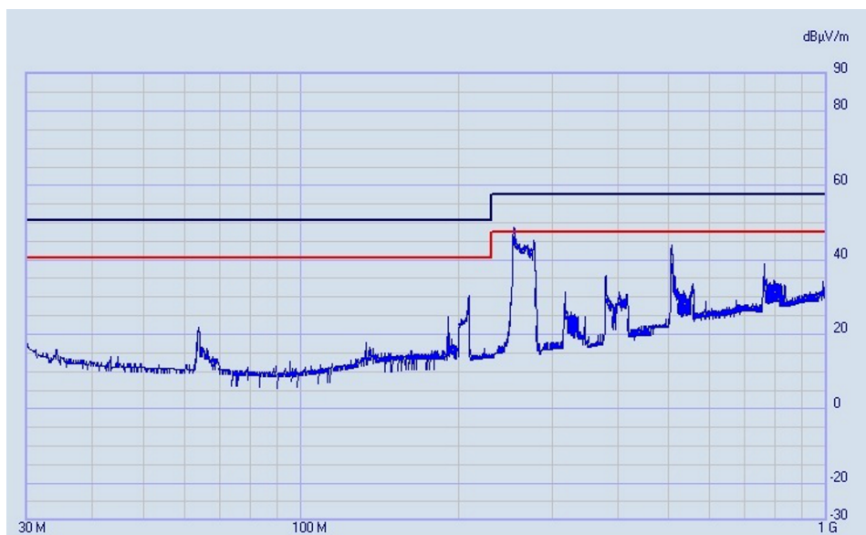
Figure 16. Radiated Emission Plot for ISOW7841-Based BIM at 3 m
