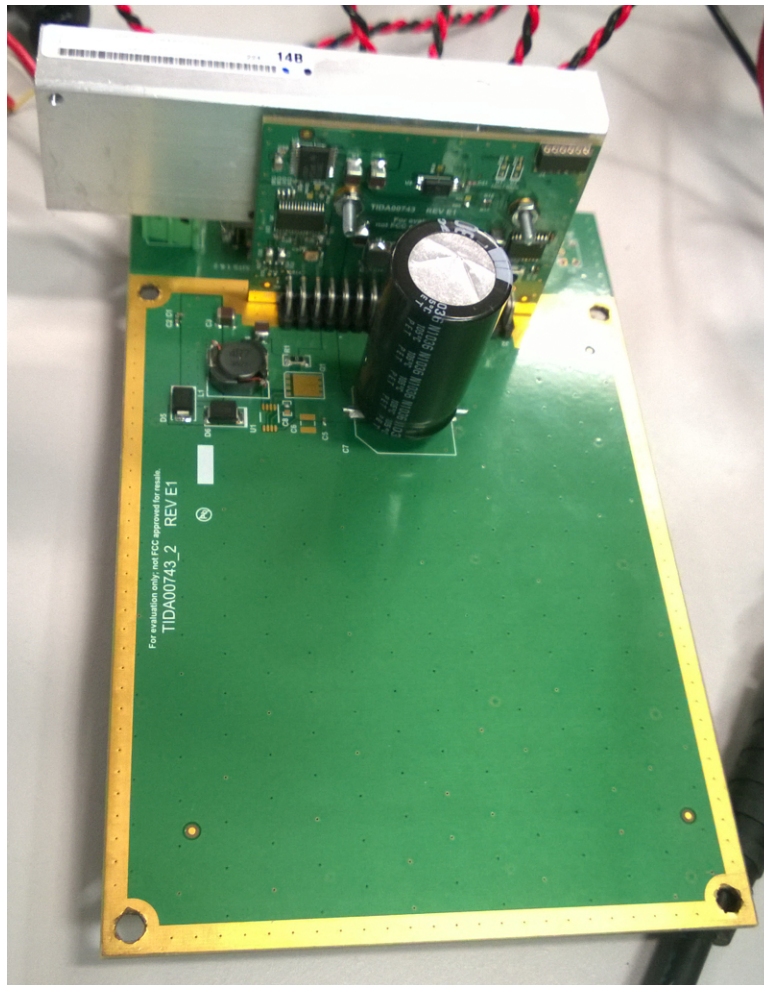
図 15. TIDA-00743 Module Board With Heat Sink Attached to Carrier Board
