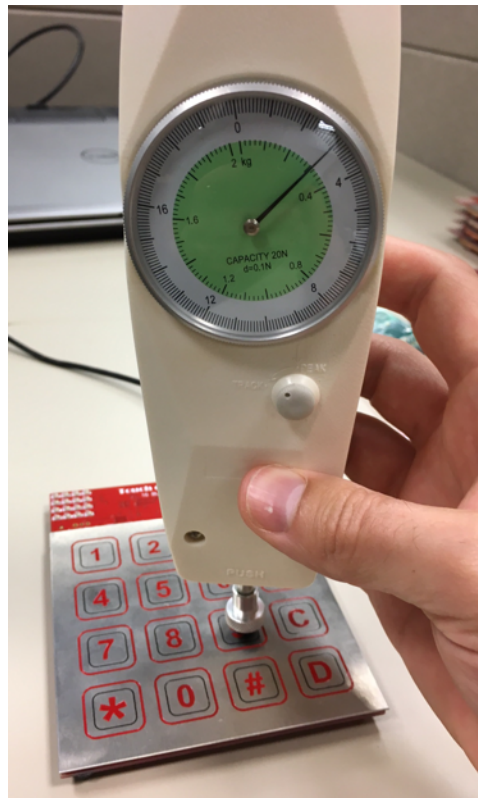
Figure 32. Test Setup With Newton Meter to Check TIDA-01102 Response to Known Forces
