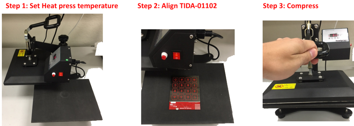
図 31. Example Compression Technique Using Heat Press
