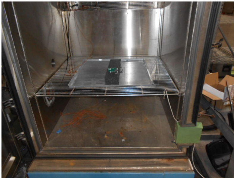
Figure 20. Wireless PIR Motion Detector Temperature and Humidity Test Setup
