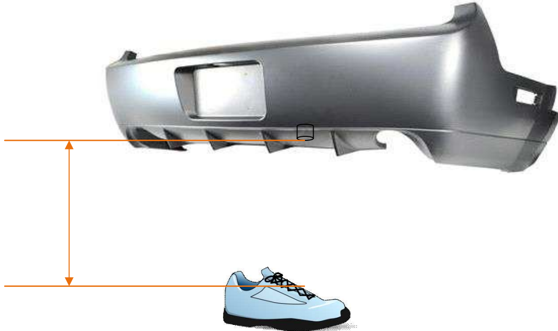
図 27. Vertical Distance Measurement From Ultrasonic Transducer to Shoe
