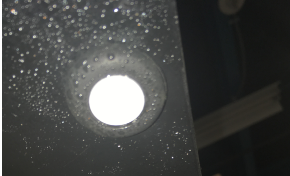
Figure 54. Water Applied to Bumper Cover and Ultrasonic Sensor
