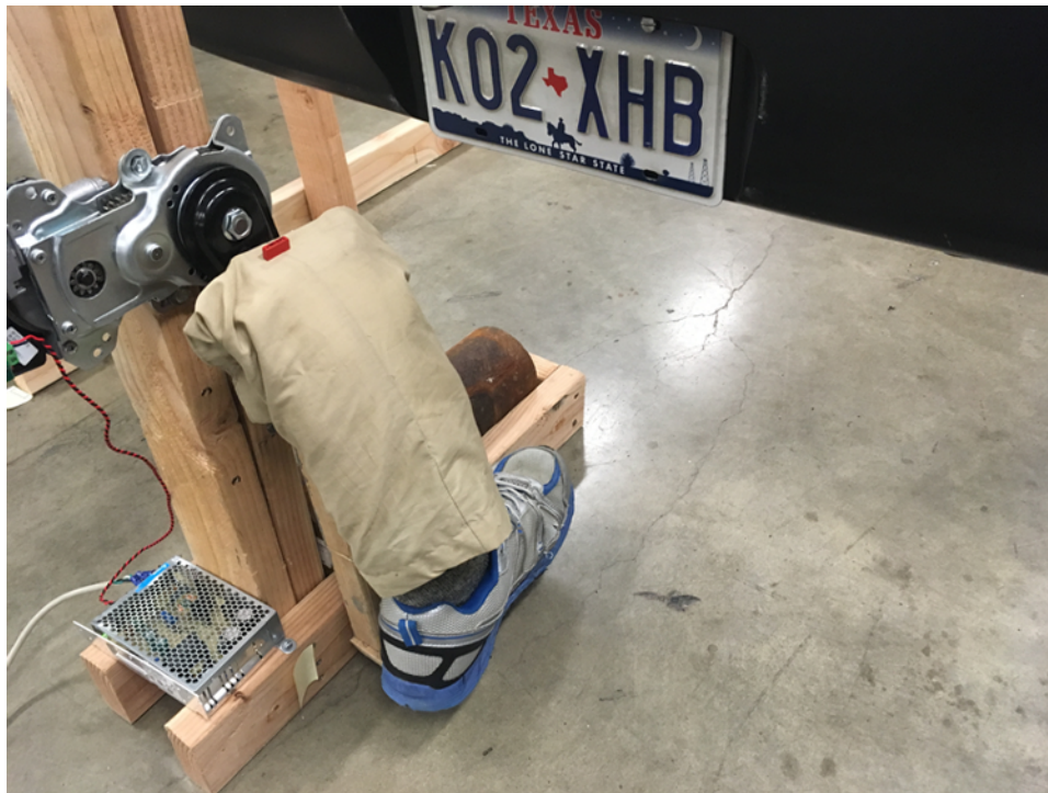
図 16. Kicking Mechanism Used for Testing
