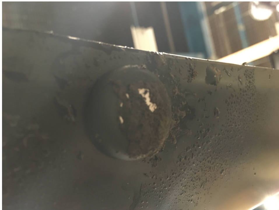
☒ 59. Mud on Ultrasonic Transducer
