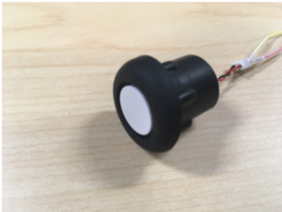
Figure 11. Closed-Top Murata Ultrasonic Transducer in Rubber Mounting Sleeve
