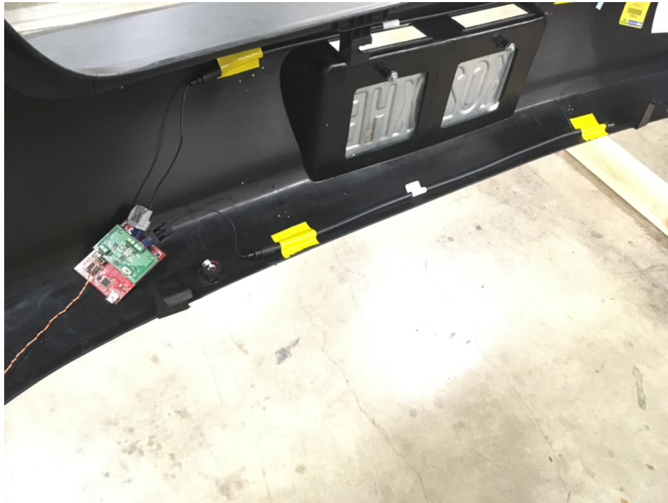
図 20. Capacitive Antennas Mounted on Bumper Cover
