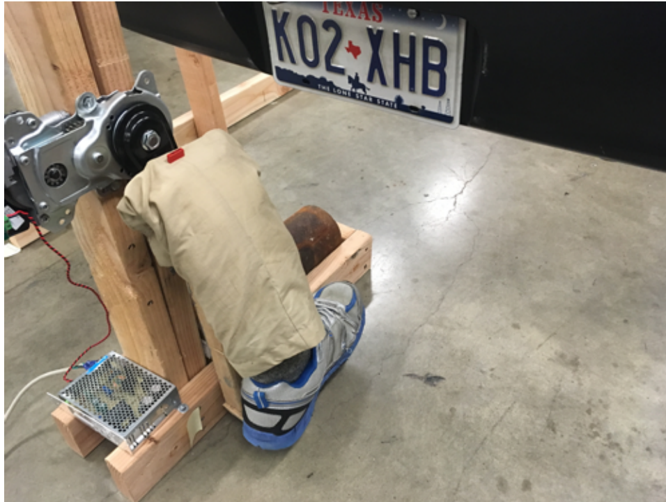
図 19. Kicking Machine With Sports Shoe
