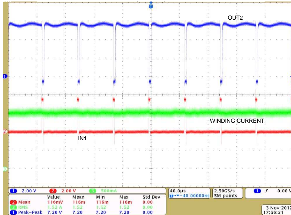
図 21. Load Test Results at 6.5-V DC Input, 1.5-A RMS Winding Current, 95% Duty Cycle
