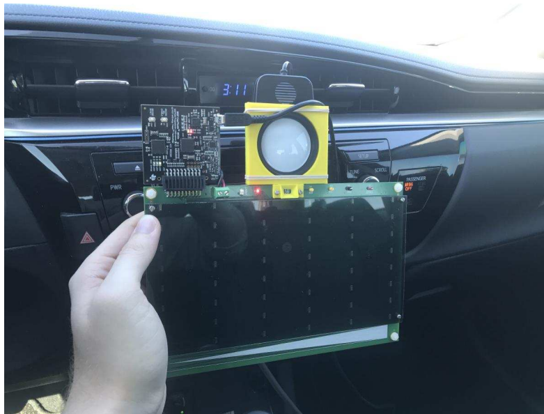
図 32. TIDA-01008 Outdoor Brightness—Center Stack Display in Vehicle
