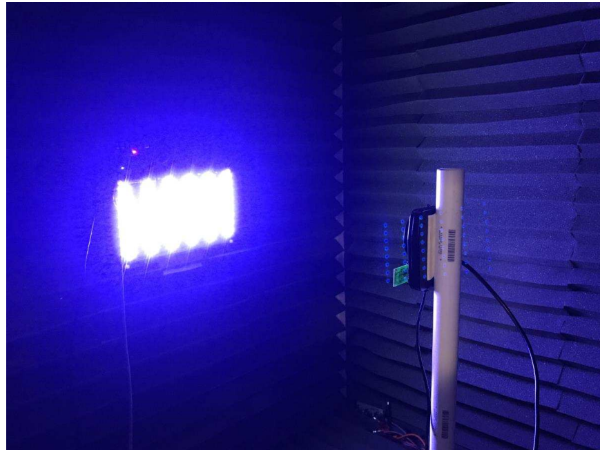
Figure 30. TIDA-01008 Illuminance Sensing Testing
