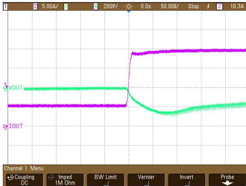
図 9. Load Transient Response
