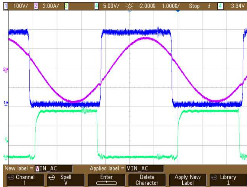
Figure 13. LLC Stage MOSFET Switching Waveform
