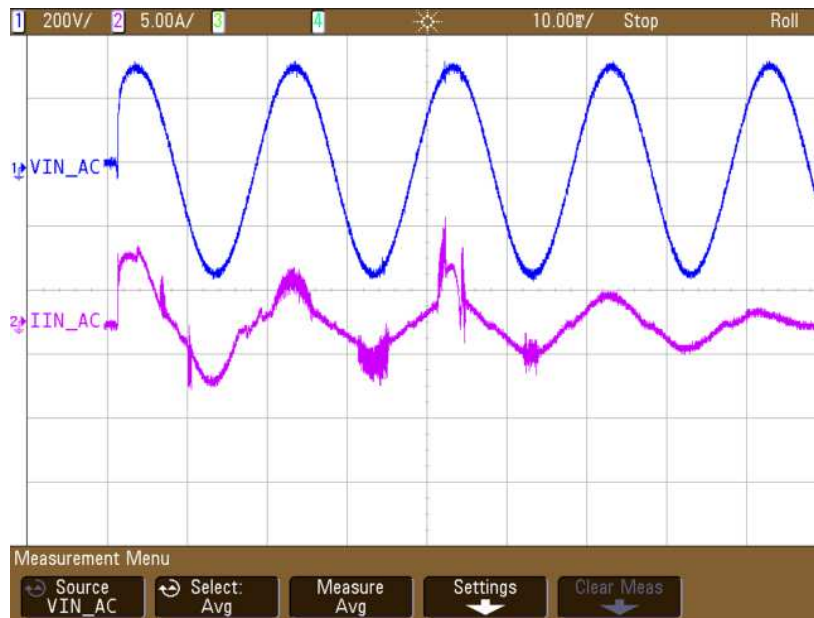
Figure 7. Inrush Current Limiting at Start-Up
