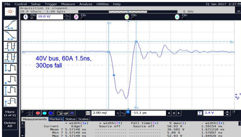
Figure 13. V_{DS} for 1.5-ns Pulse With 40 V of Bus Voltage
