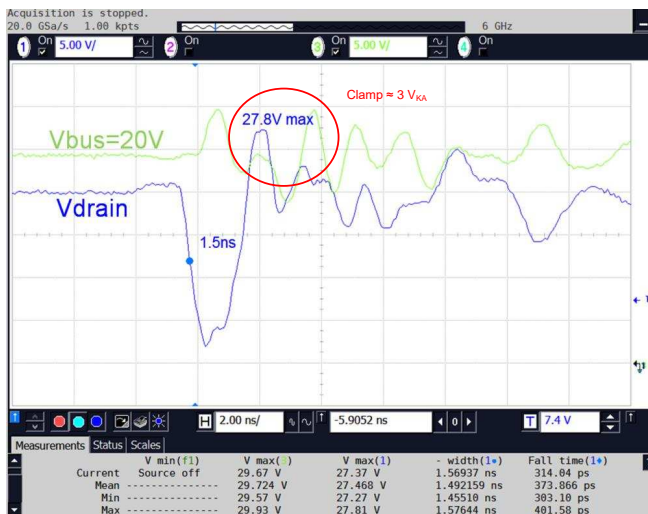
8. Overshoot Voltage With Clamping Diode
