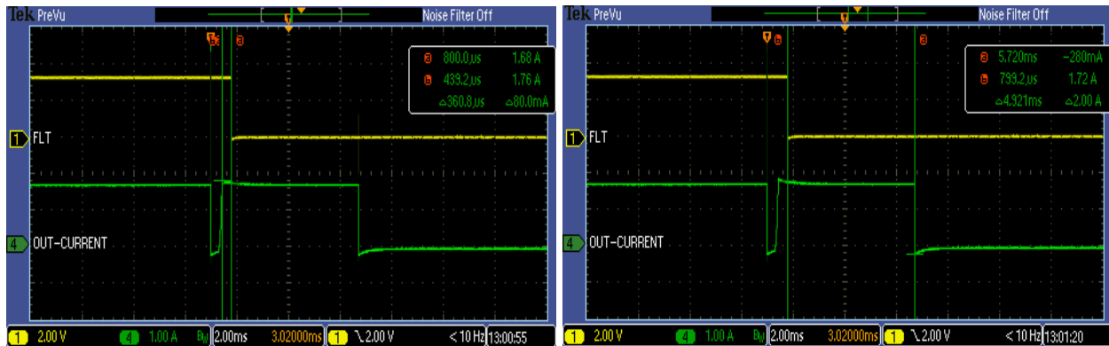
Figure 22. Short-Circuit Event Under Normal Operation of TPS26600
