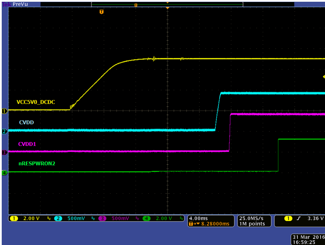
Figure 7. Power-On Sequence for the TPS65911x With nRESPWRON2
