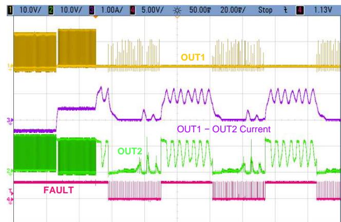
Figure 39. DRV8847 – OUT1 to GND Short During Motor Running
