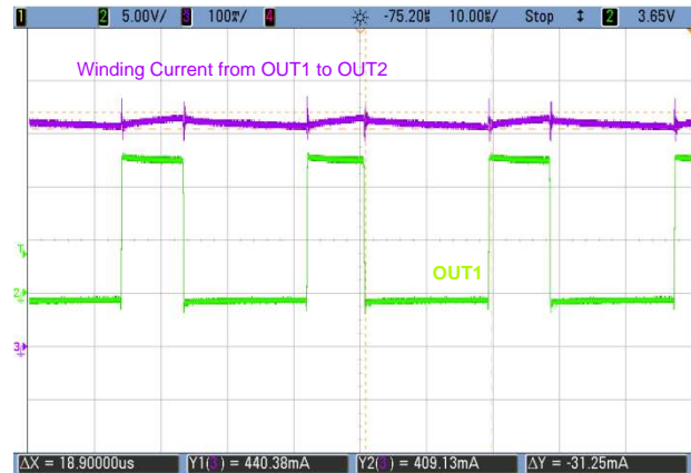
図 28. Current Regulation With Slow Decay Mode
