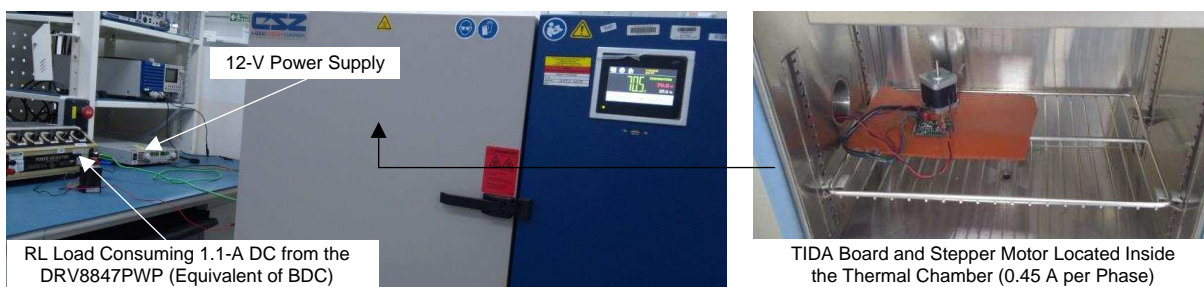
図 45. Setup for Testing the Design at Multiple Ambient Temperatures
