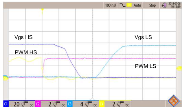
図 20. Six Mode PWM vs V_{GS} LS and HS, Phase A Current at 48 V, -5 A Soft Switching
