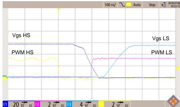
図 24. Independent Mode PWM vs V_{GS} LS and HS. Phase A Current at 48 V, -5 A Soft Switching
