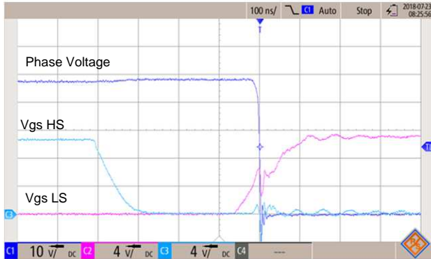
図 10. Hard Switching Phase A Voltage Falling Edge, Phase Current at 48 V, 10 A
